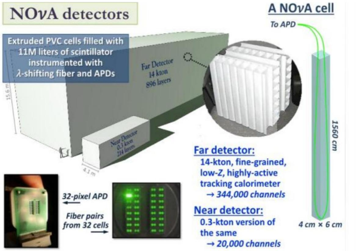
Figure 2. General concept of the NOvA detectors design
