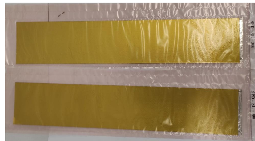
Photo of SPD-300-2 signal layers (n+ side) at top; Shielding layers at bottom
