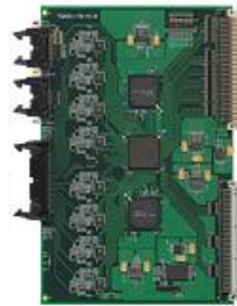
TQDC16 (16-channel time and charge digitizer)
