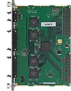
TQDC16 (16-channel time and charge digitizer)
