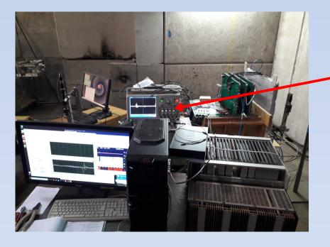
**Readout:** Oscilloscope DPO 1GHz CF (250ps) & GSI-amplifier (~1GHz)
