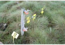
$\rm NH_3$  released from a 10 m pipe at 1 m height when wind direction is 180–215° and speed is 2.5 m s<sup>-1</sup>  $\rm NH_3$  concentrations measured by passive samplers (ALPHA)
