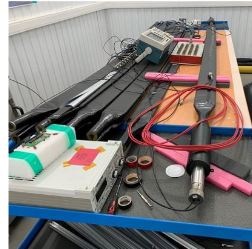
Trigger system – ten 10 \times 200 \text{ cm}^2 scintillation detectors
