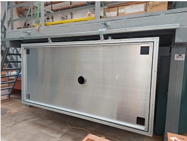
Scint. Wall with a beam hole for heavy ion (additional quartz hodoscope is planned to be placed at the center)
