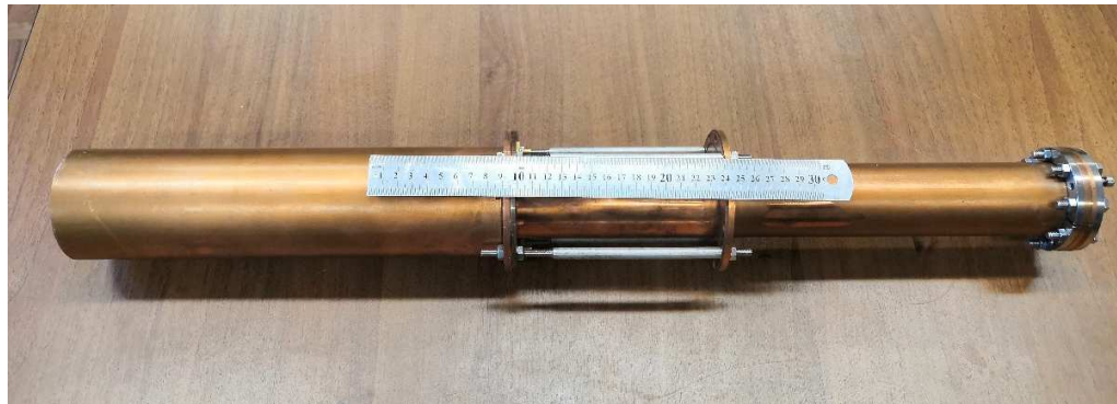
Fig. 3. Cavity system for ordering the monochromatic positron flow.
