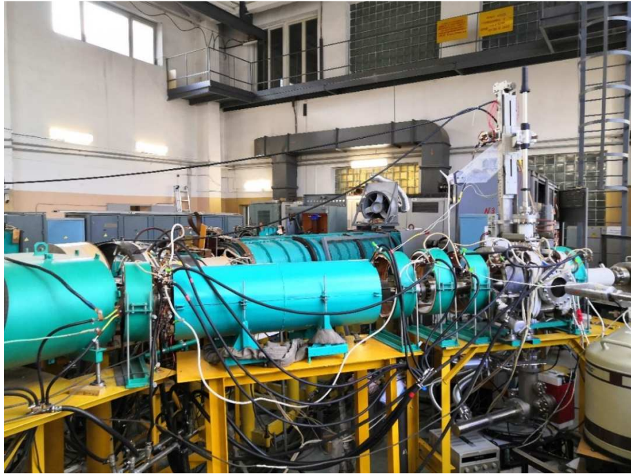
Fig. 2. Specialized channel of the slow-positron beam.
