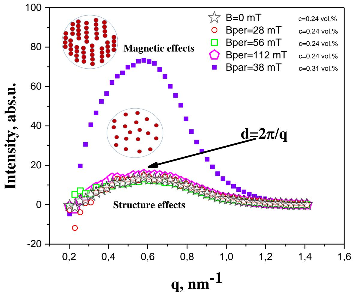
Determination of an average distance  $d \sim 10.8 \text{ nm}$  between the elongated clusters in the ME polymerized in magnetic field applied parallel to the sample plane !
