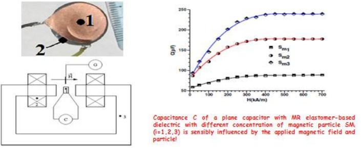
Capacitance  $C$  of a plane capacitor with MR elastomer-based dielectric with different concentration of magnetic particle  $S_m$  ( $i=1, 2, 3$ ) is sensibly influenced by the applied magnetic field and particle!
