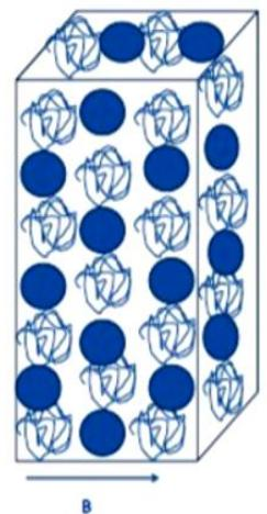
SANS data indicates that in the case of MEs polymerized under the magnetic field the blobs are preferably elongated in the direction normal to the field.
