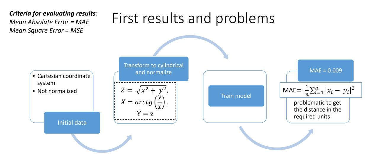
The neural network model obtained at the previous stage predicted the primary event vertex with MAE = 0.009. The problem is that the error was calculated for normalized data, and it turned out to be quite problematic to get the distance in the required units.
