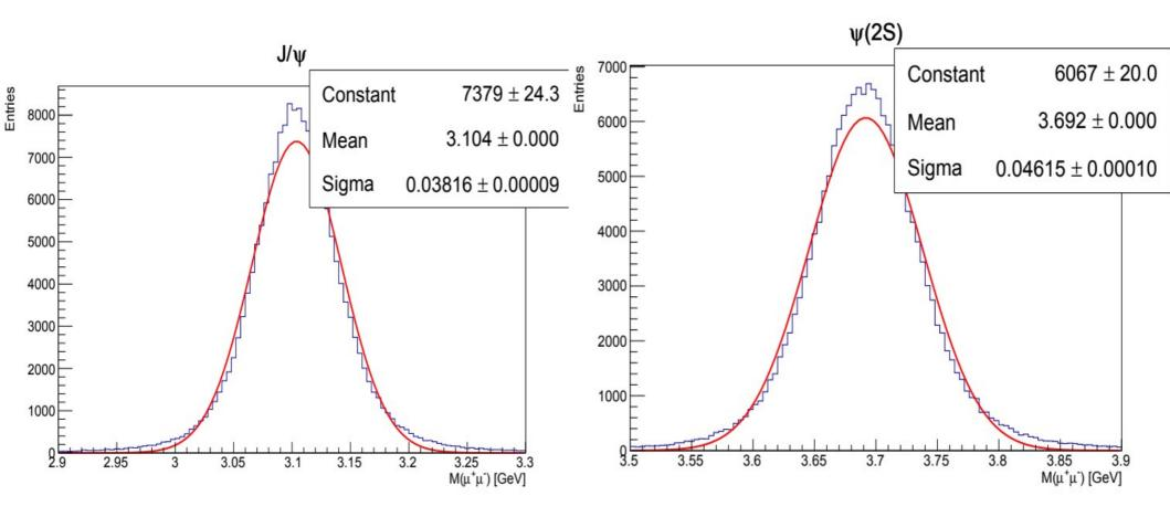
Integral dimuon mass resolution for J/ $\psi$  and  $\psi$ (2S).
