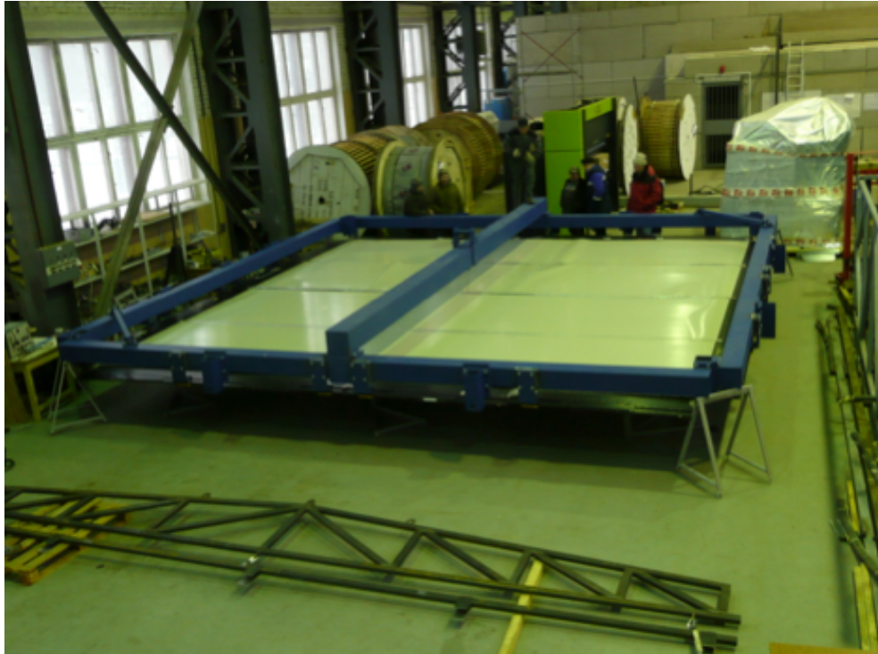
Fig.3.3.4 The TT wall prototype at JINR for mechanical tests and elaboration of the assembly procedure. Auxiliary tools designed for the TT assembly are also shown.
