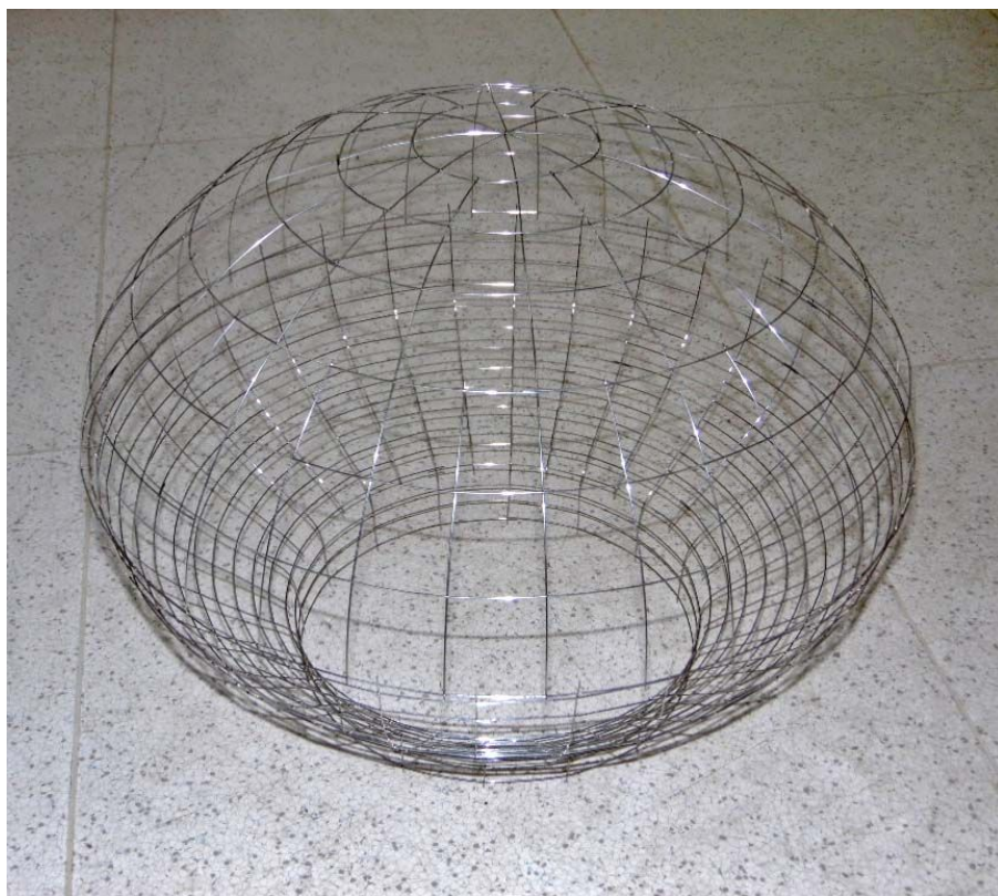
Fig.3.5.3. The prototype of the EMF screen produced by DLNP workshop.
