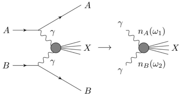
$$\sigma(AB \rightarrow ABX) = \int_0^\infty d\omega_1 \int_0^\infty d\omega_2 \sigma(\gamma\gamma \rightarrow X) n_A(\omega_1) n_B(\omega_2)$$
