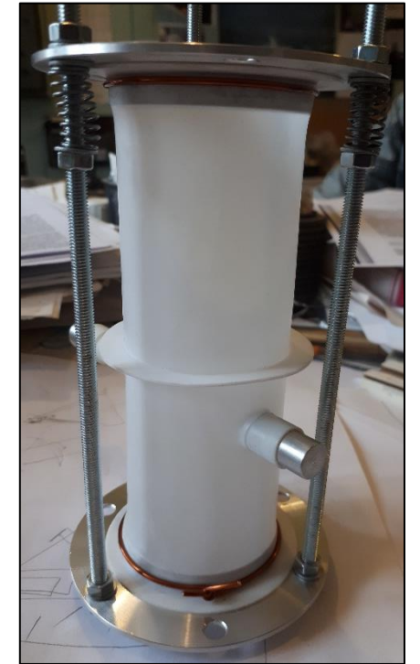
Fig. 10. The first example of the PTFE cylinder with the converter tube.
