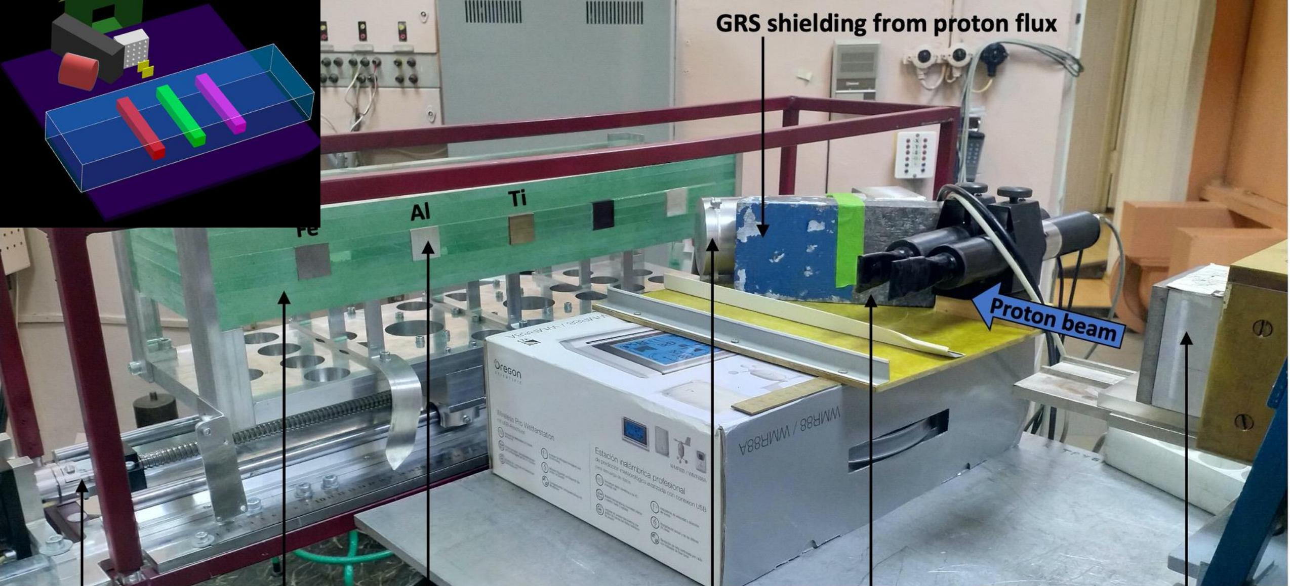
GRS shielding from proton flux
