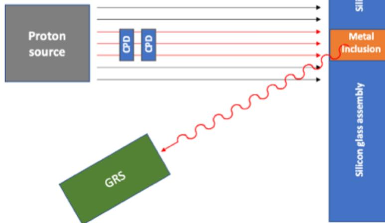
GRS = Gamma-ray spectrometer; CPD = Charge particle detector
