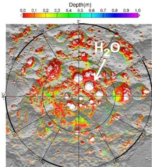
Water distribution in regolith according to LPNS data from Lunar Prospector (NASA)
