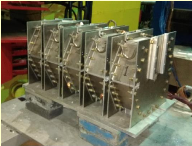
QUINTA set-up without lead shielding
