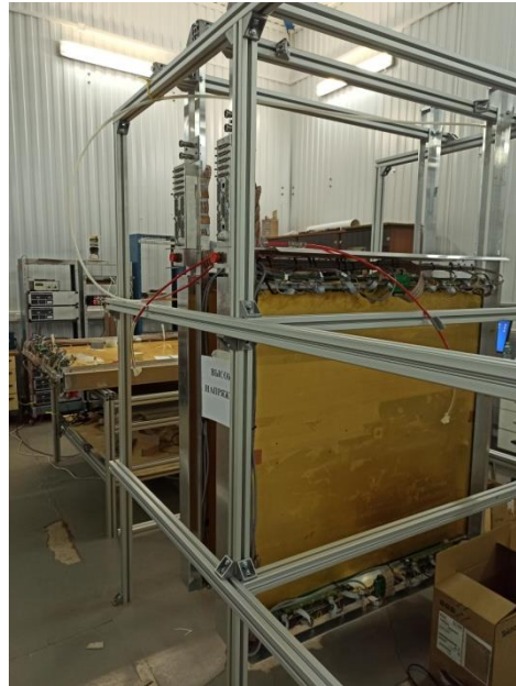
Cosmic stand for the 1065 \times 1065 \text{ mm}^2 CSC
