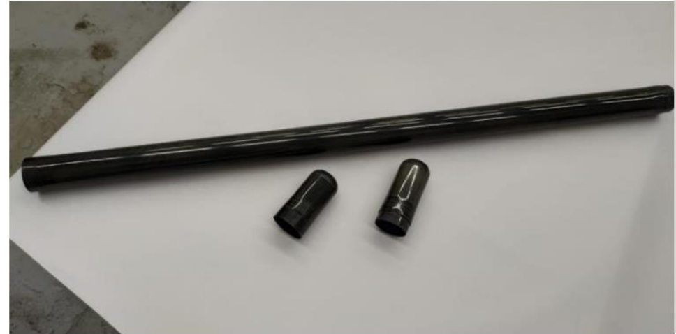
1 meter prototype of the BM@N carbon beam pipe (DD "Arkhipov")
