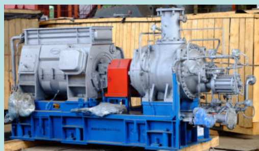
Helium screw compressors "Kaskad-110/30"
