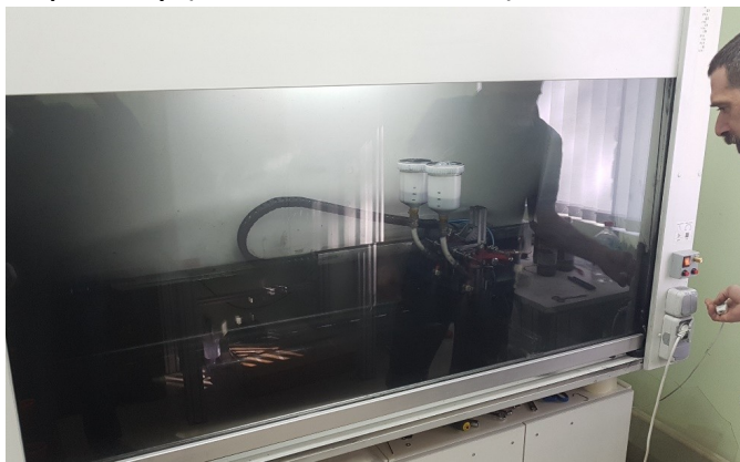
Automatic painting of the conductive layer on the glass
