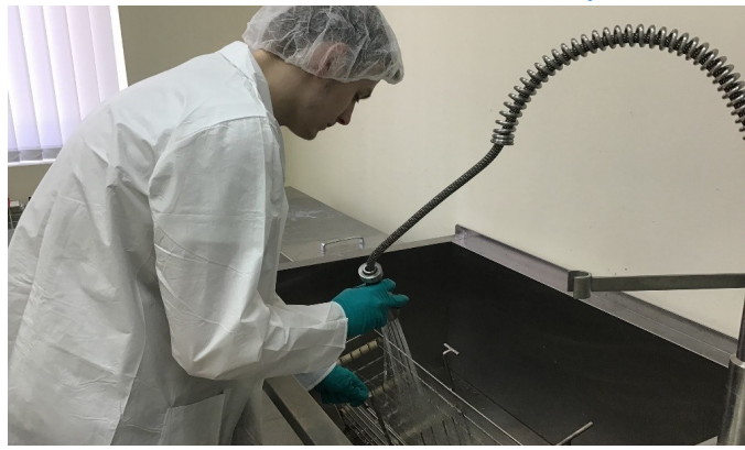
Glass cleaning with ultrasonic wave & deionized water
