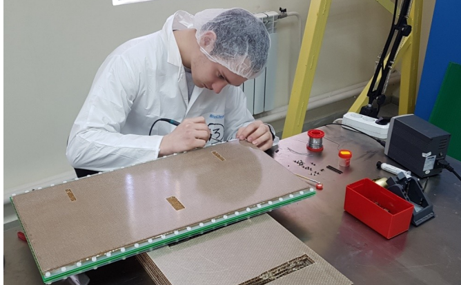
Soldering HV connector and readout pins
