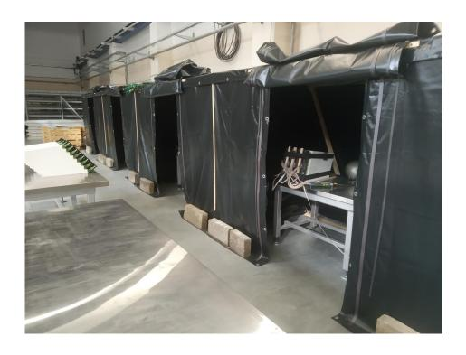
Test area is ready for the mass tests of modules by means of cosmic muons
