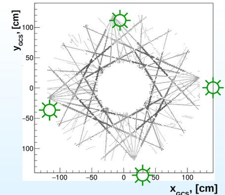
On 4 planes perpendicular to Z inside the TPC camera from 4 points, there are 7 rays, the projections of which intersect all sectors.
