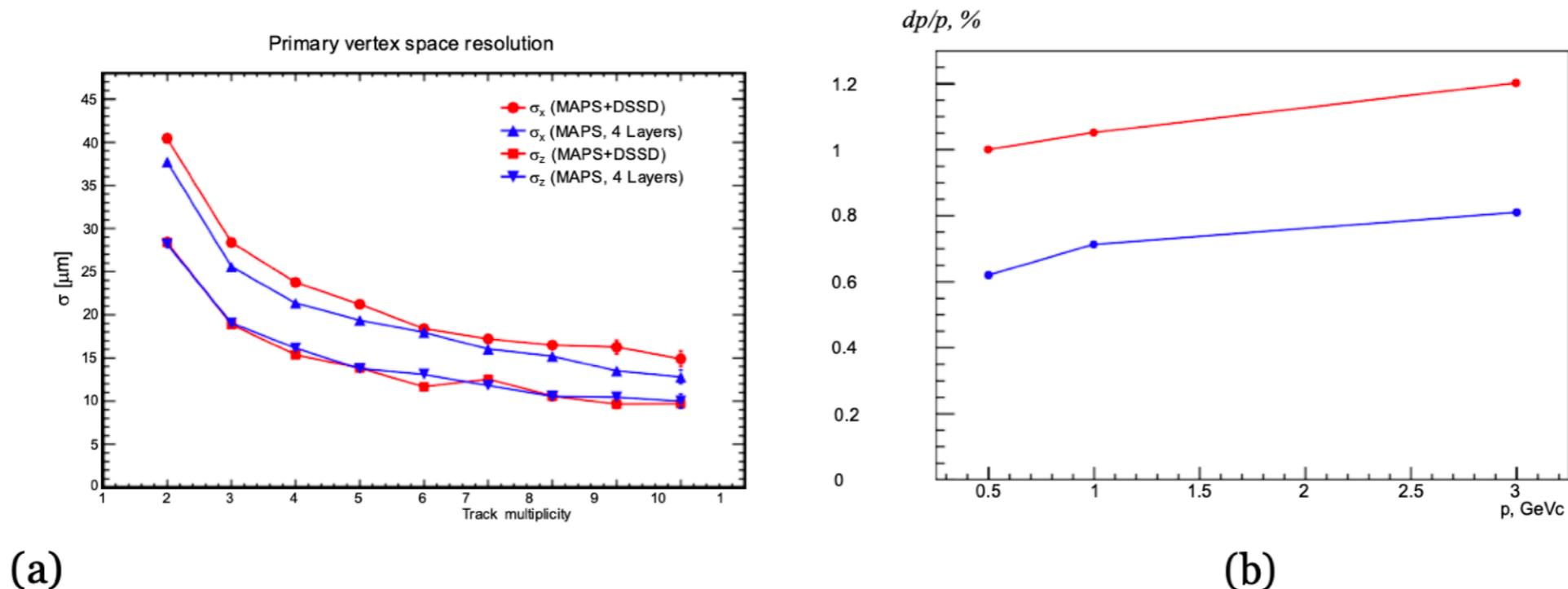
Figure 3: (a) Vertex position resolution as a function of track multiplicity and (b) momentum resolution as a function of particle momentum for the VD consisting of 3 MAPS+2 DSSD and 4 MAPS, respectively.
