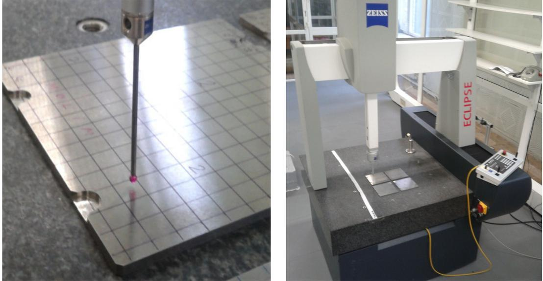
Figure 7: Measurement of the geometric parameters of the FCAL tungsten absorber plates using Zeiss Eclipse three-axis coordinate measuring machine.
