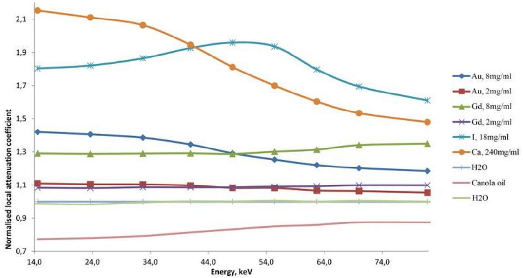
Figure 28: Dependence of linear attenuation coefficient on energy for various substances (normalized to water).
