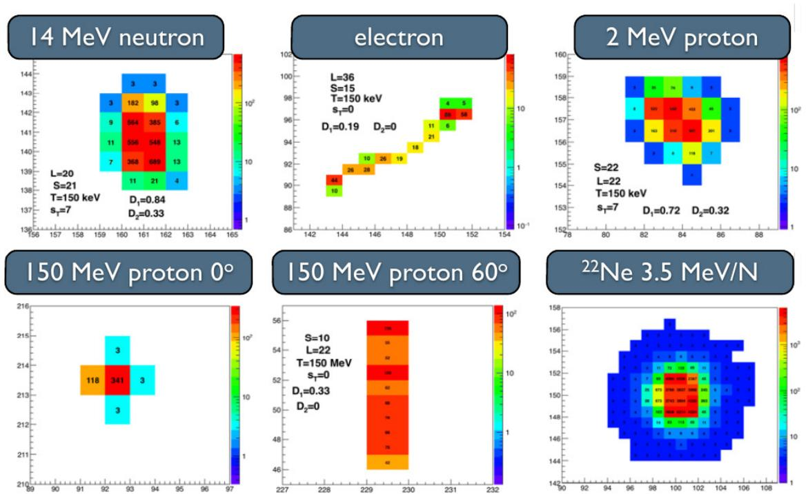
Figure 16: Typical clusters formed in Timepix detectors by different types of particles.
