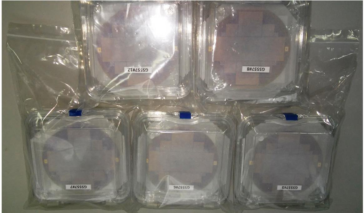
Figure 9: The first batch of GaAs:Cr sensor wafers with a diameter of 102 mm, produced within the GALAPAD-2 project.
