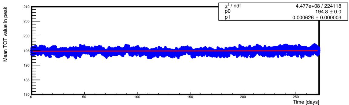
Figure 12: Change in the position of the 59 keV photopeak of an  $^{241}\text{Am}$  source as a function of time.
