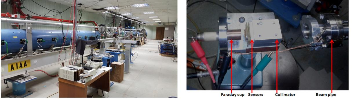
Figure 2: The output beam-line of the Linac-200 accelerator and the setup for irradiating pad sensors.
