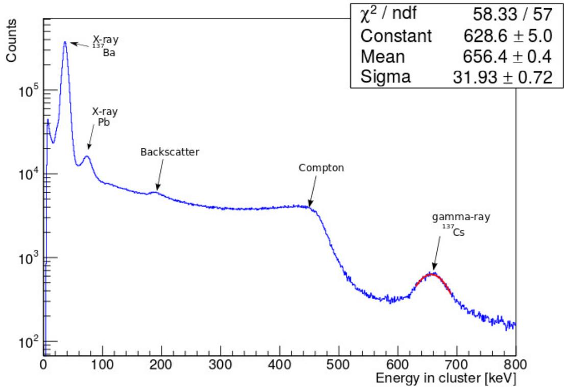
Figure 11: Spectrum of  $^{137}\text{Cs}$  after the per-pixel energy calibration of the Timepix detector with 1 mm thick gallium arsenide sensor.
