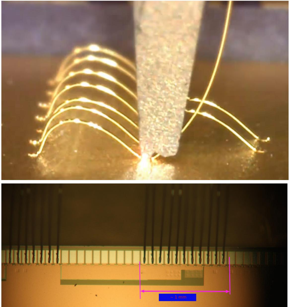
Figure 24: An example of creation of micro-wire connections by the “wedge-wedge” method (above) and an example of the connections of the Medipix chip to a chipboard (below).
