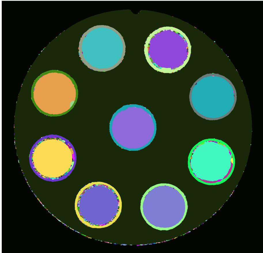
Figure 27: Segmented cross-section of phantom for 9 thresholds.
