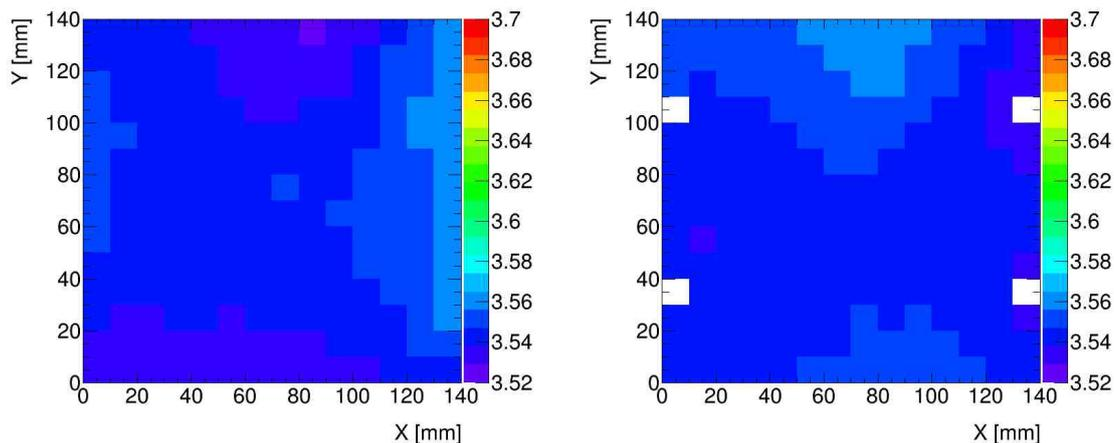
Figure 8: Results of measuring of the surface shape of the tungsten absorber plates for FCAL. The distance to the surface of the plate in mm is shown relative to the base plane for the two sides of the absorber plate.
