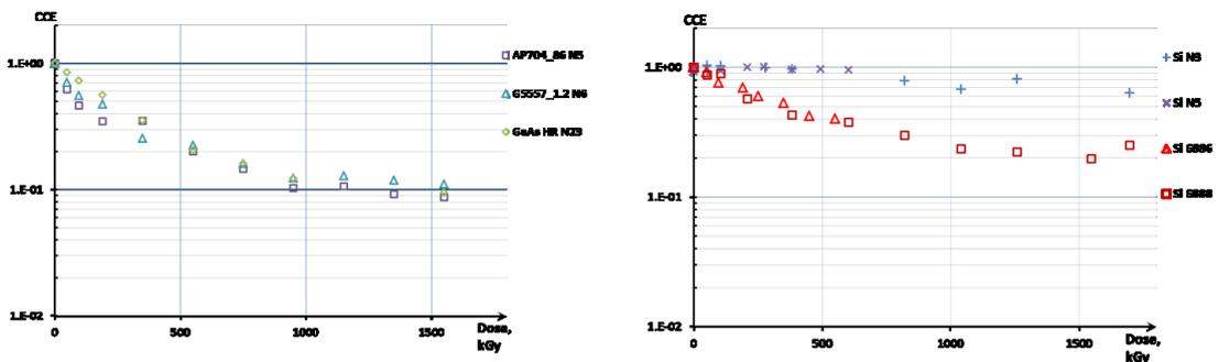
Figure 4: Dependence of the charge collection efficiency on the absorbed dose. Left - gallium arsenide detectors, right - silicon detectors.
