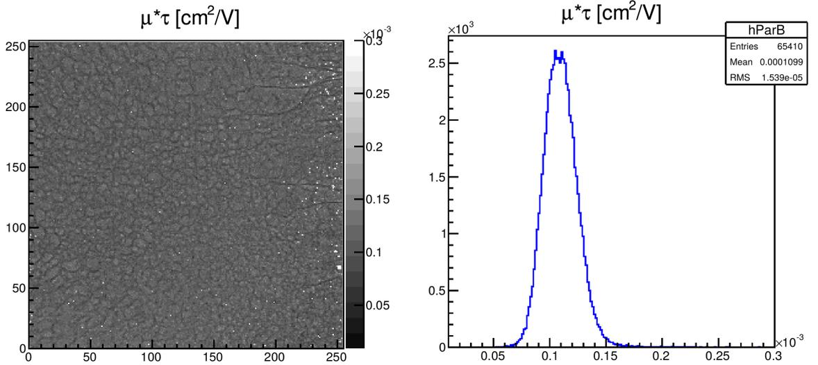
Figure 14: The value of  $\mu\tau$  depending on the pixel position (left); distribution of the  $\mu\tau$  values for all pixels in the detector.
