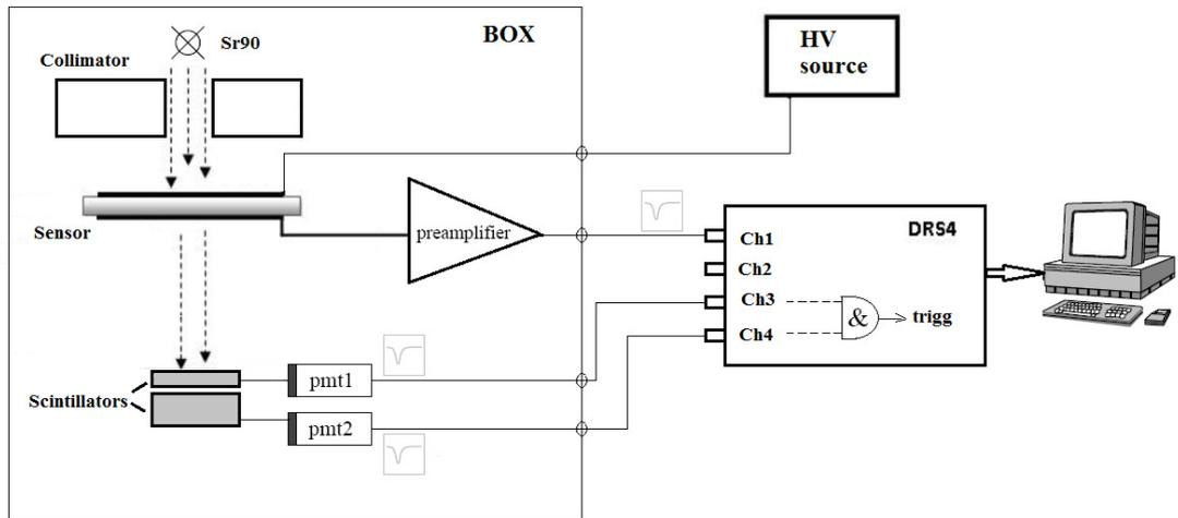
Figure 22: Station for measuring charge collection efficiency.
