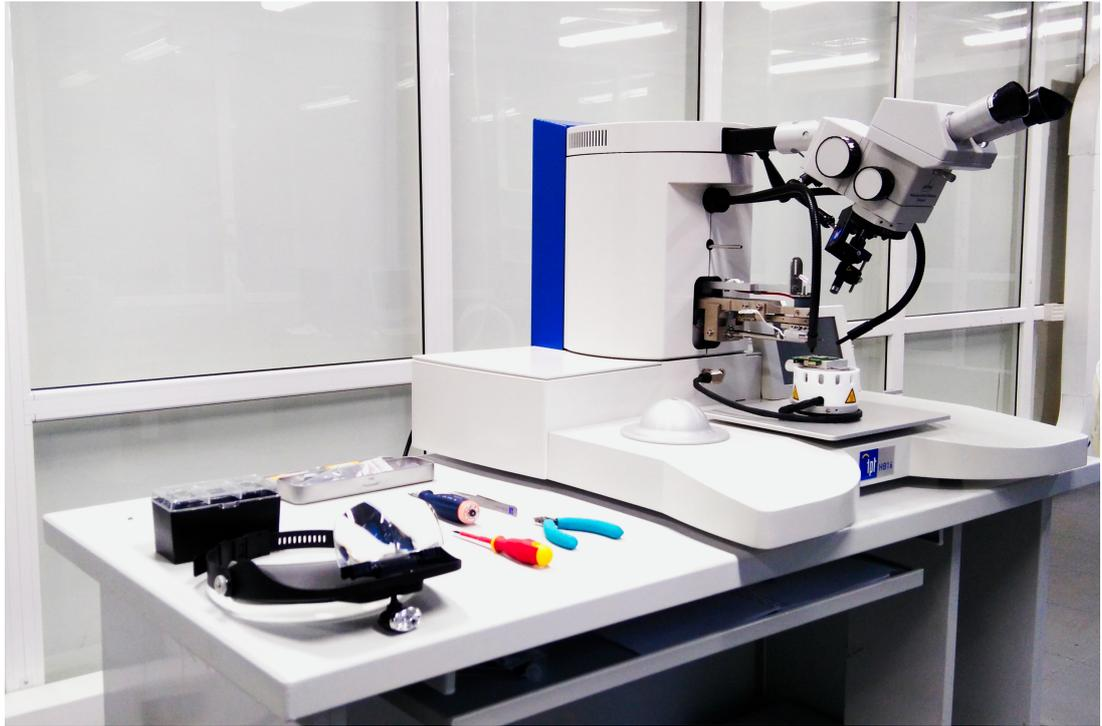
Figure 23: Installation for ultrasonic microwelding.
