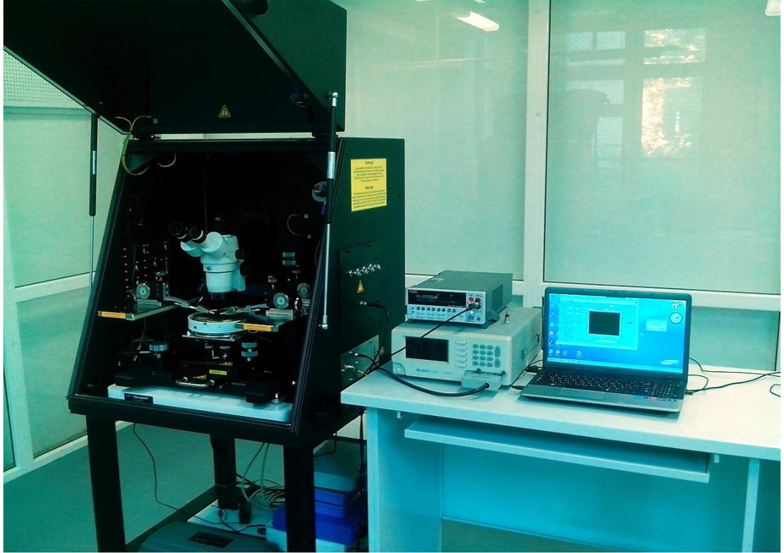
Figure 21: Testing bench based on the Cascade Microtech EPS150TESLA probe station for studying properties of semiconductor materials.
