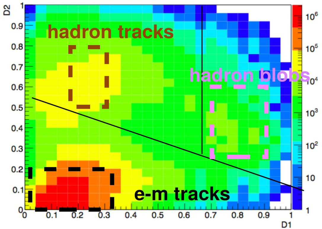
Figure 17: Separation of cluster types in the Timepix detector based on parameters D1 and D2.
