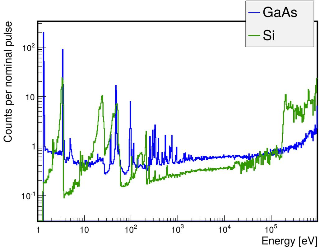
Figure 18: Spectrum of neutrons in Timepix detectors with sensors from silicon and gallium arsenide.
