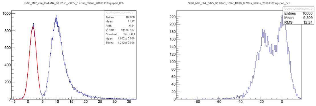
Figure 5: The spectra obtained on gallium arsenide (left) and silicon (right) detectors after irradiation with a dose of 0.5 MGy, at room temperature.
