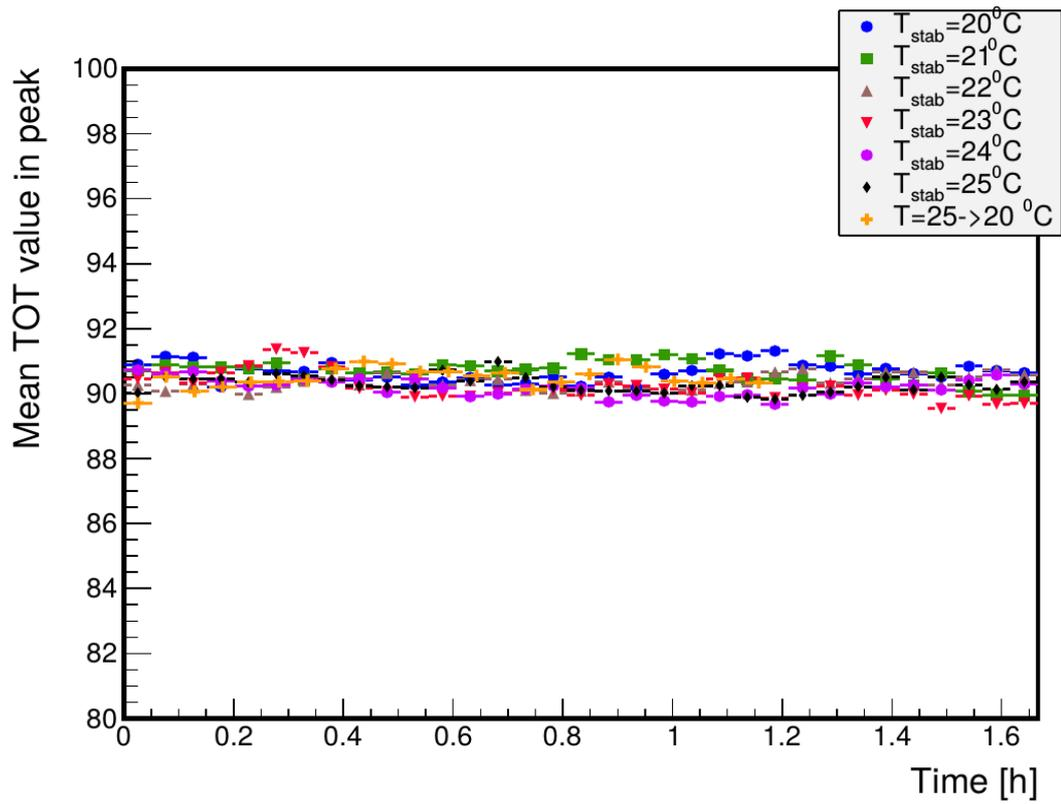
Figure 13: Stability of the position of the 59 keV photopeak of an  $^{241}\text{Am}$  source at different temperatures.
