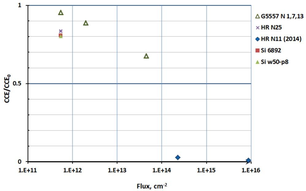
Figure 6: Dependence of the relative efficiency of charge collection on neutron fluence for silicon and gallium arsenide detectors.
