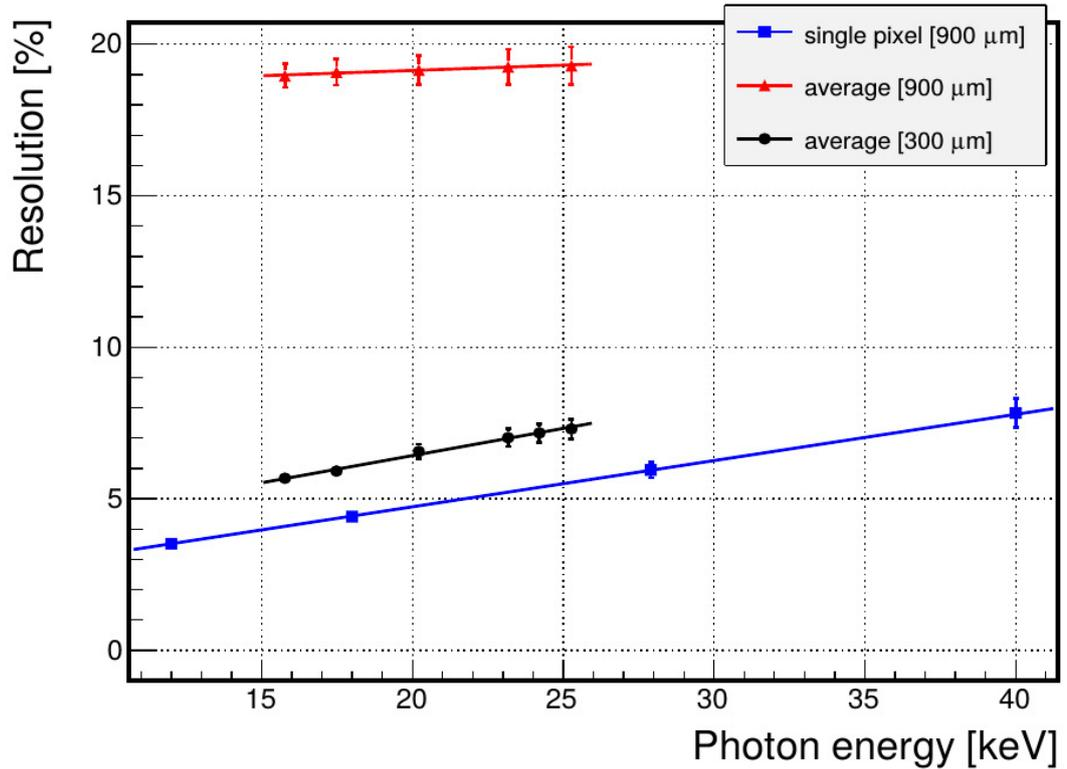
Figure 15: The dependence of the energy resolution of the detector (expressed as a percentage of the measured energy) on the photon energy.
