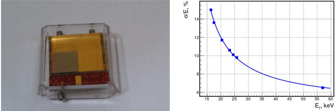
Figure 10: General view and energy resolution of the Timepix detector with 1 mm thick gallium arsenide sensor.
