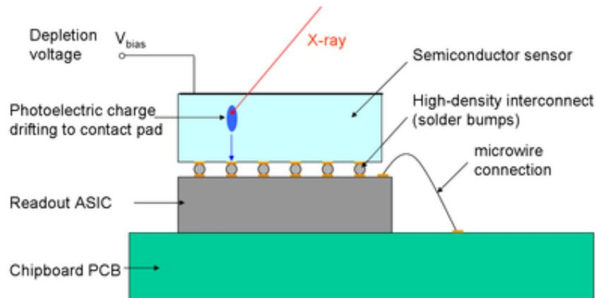
Figure 1: Typical scheme of a hybrid pixel detector.
