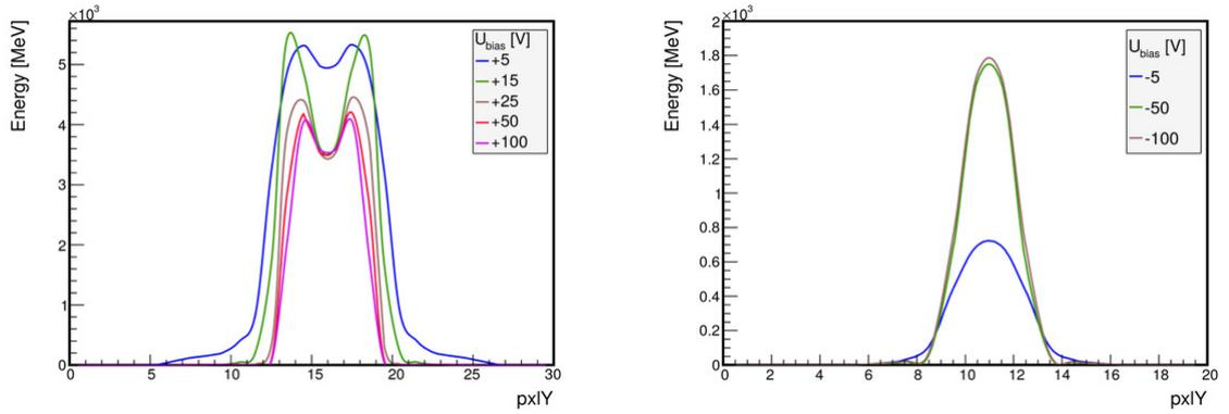
Figure 19: “Volcano effect” in the silicon (left) and gallium arsenide (right) Timepix detectors when irradiated with Ne ions with an energy of 158 MeV.
