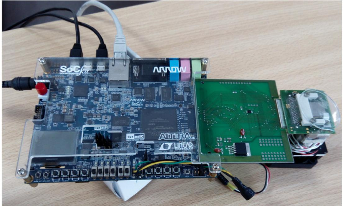
Figure 26: The prototype of the readout electronics unit for the Medipix family detector.
