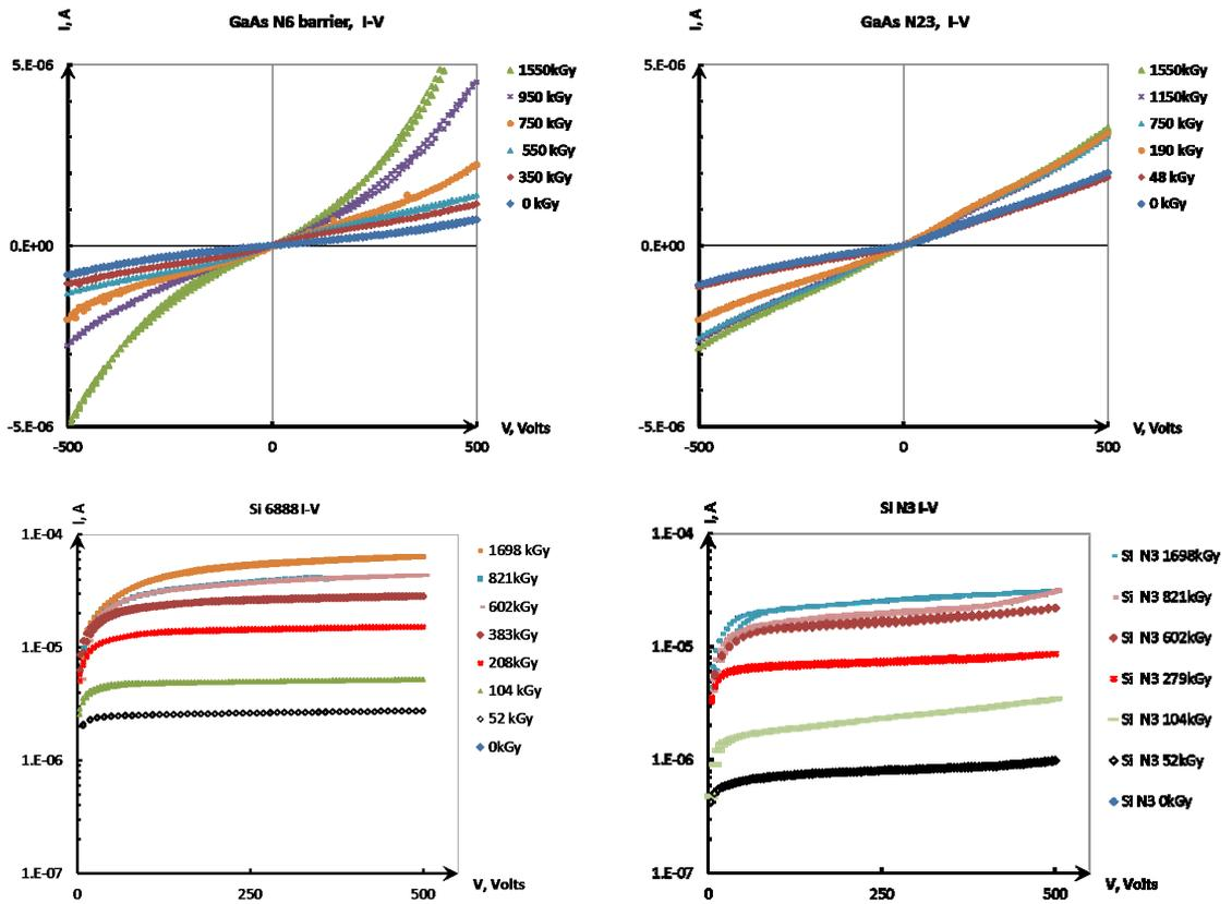
Figure 3: Current-voltage characteristics of detectors after irradiation. The upper row are gallium arsenide detectors (resistive structures on the left, barrier structures on the right), the lower row are silicon detectors (n-type silicon detectors from USCS (USA) on the left, the detectors provided by N. I. Zamyatin's group on the right).
