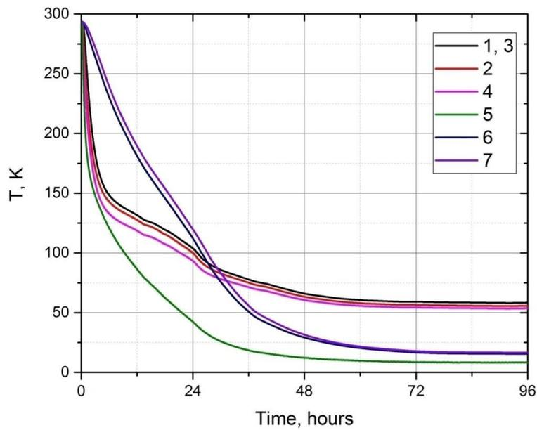
**Fig. 4.4.** Graphs of temperature in various parts of the cryostat versus time. Temperature of magnet – 6, 7; temperature of warm ends of HTSC current leads – 1, 3; temperature of second stage of cryorefrigerator – 5, temperature of first stage of cryorefrigerator – 2, 4.
