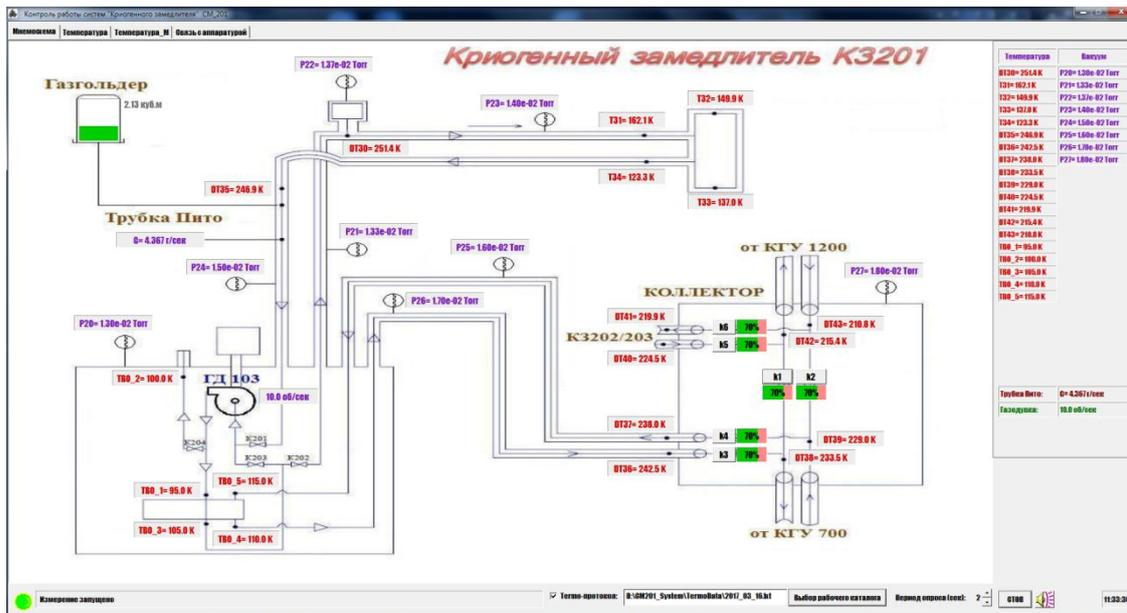
Fig. 7.4. New graphic interface for CM-201 cold moderator.
