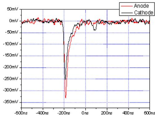
**Fig. 5.7.** Shape of anode and cathode signals (filling gas –  $\text{CF}_4$  at 1 atm.).
