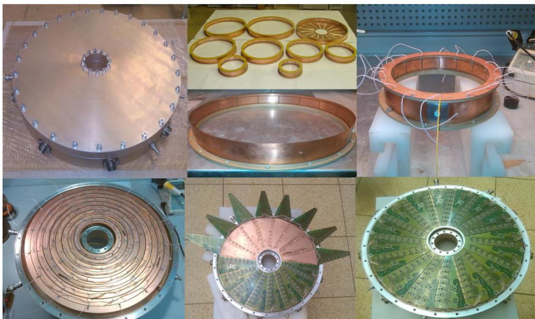
**Fig. 5.2.** Photos of the housing (left), internal part of the detector and 9 independent coaxial rings (right).
