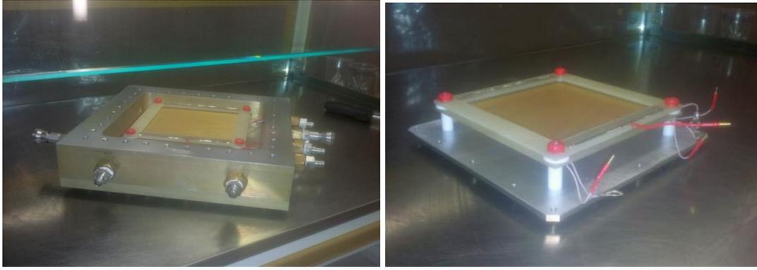
**Fig. 5.6.** Prototype of PSD with  $^{10}\text{B}$  converter (left). Electrode system of prototype (right).
