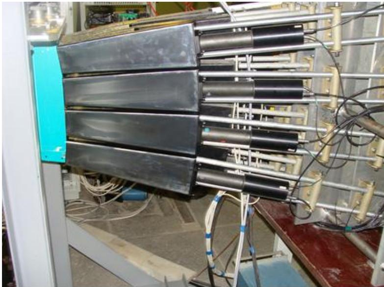
**Fig. 5.8.** Scintillation counters of section 4 of the ASTRA detector, which are installed on the FSD diffractometer.
