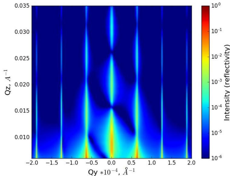
**Fig. 2.2.** Simulation of a full reflectometric experiment in the modified kinematic approximation of the system of gold columns on a silicon substrate.
