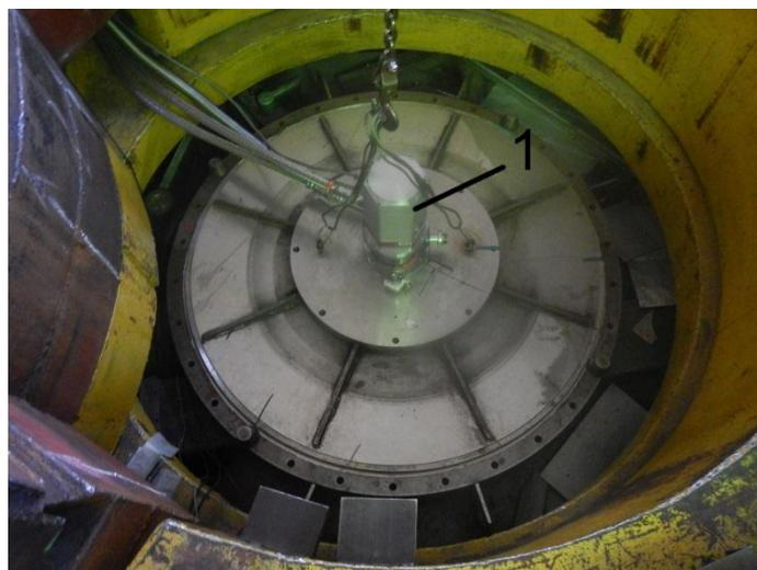
**Fig. 4.5.** Photo of cryostat with cryorefrigerator in the shaft of the DIN-2PI spectrometer.
