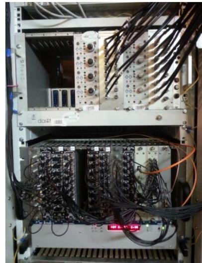
**Fig. 3.6.** Electronics of high-voltage power supply of detectors (top crate), modules of detector electronics and data acquisition electronics (bottom crate).
