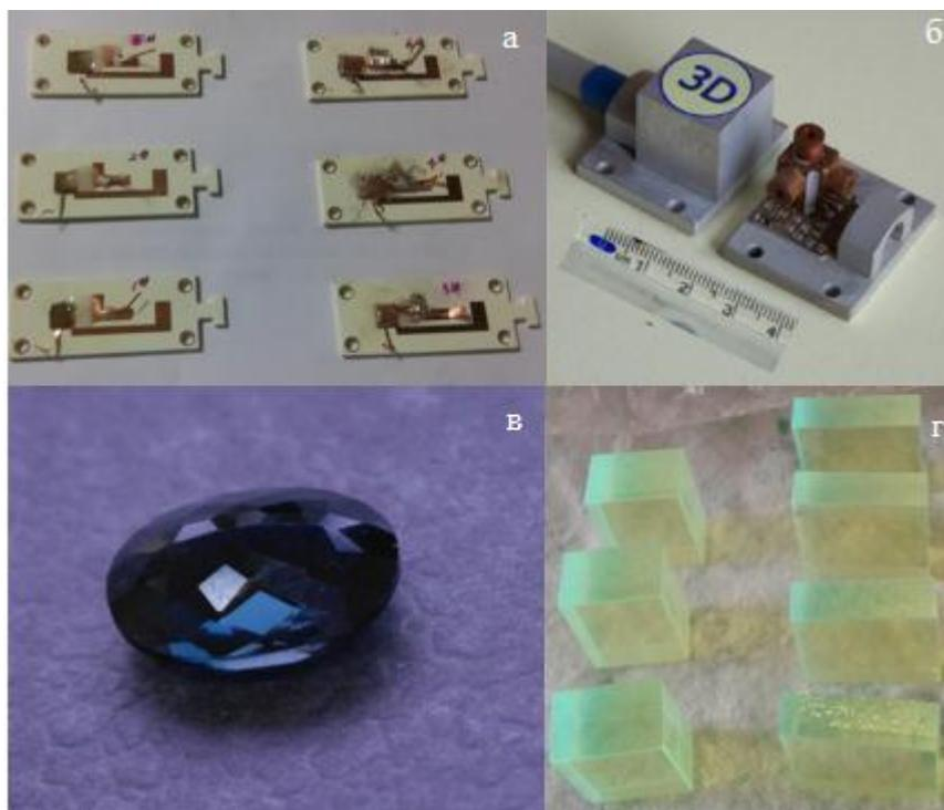
**Fig. 1.5.** Samples for the experiments conducted at the radiation research facility: a – diamond single crystal; b – magnetic 3D Hall sensors; c – topaz, d – silicon scintillators.
