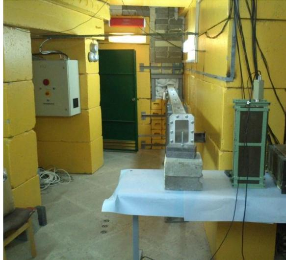
**Fig. 3.2.** Exit section of the neutron guide.
