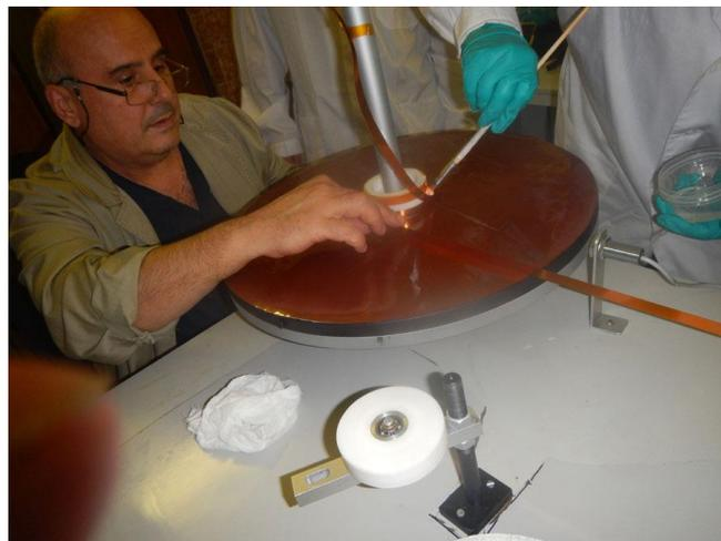
**Fig. 4.3.** Manufacturing of magnet windings on a special machine.
