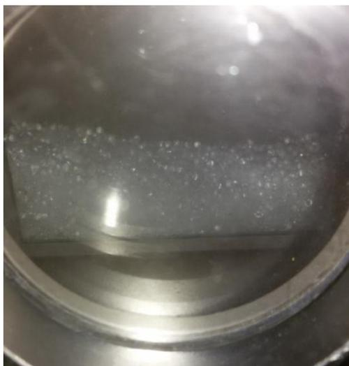
**Fig. 1.2.** Photo of the chamber during the experiment. Temperature inside the chamber is  $T = 80$  K. About 15,000 pellets (0.5 l) are loaded.
