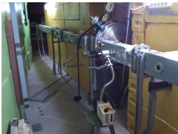
**Fig. 3.1.** Starting section of the curved neutron guide and Fourier chopper on IBR-2 beamline 13.
