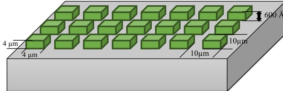
**Fig. 2.1.** System of gold columns on a silicon substrate (column height – 600 Å, column width – 4×4 μm, spacing in the horizontal plane – 10×10μm).
