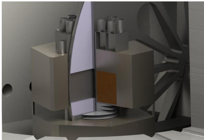
**Fig. 1.6.** Design of Np-237 based reactor.
