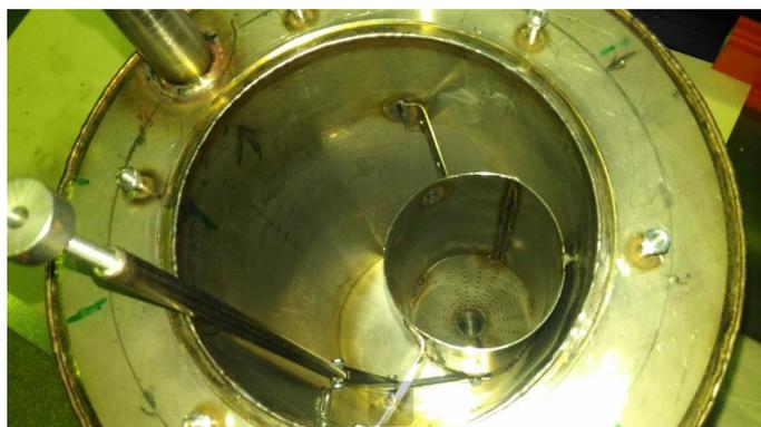
**Fig. 1.3.** A device for nitrogen-free charging of frozen pellets into the CM202 chamber.
