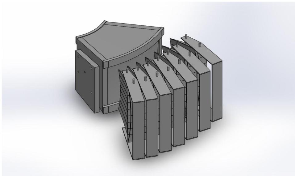
**Fig. 5.11.** 3D view of the left arm of the ASTRA-M detector.
