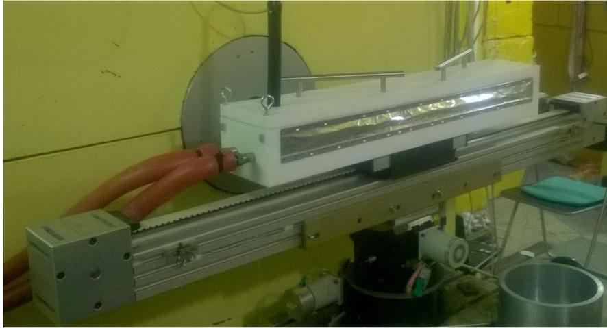
**Fig. 6.2.** Automatic sample changer for 25 samples at the YuMO spectrometer.
