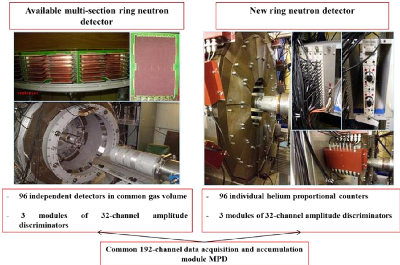
**Fig. 5.1.** New detector system of the DN-6 diffractometer.
