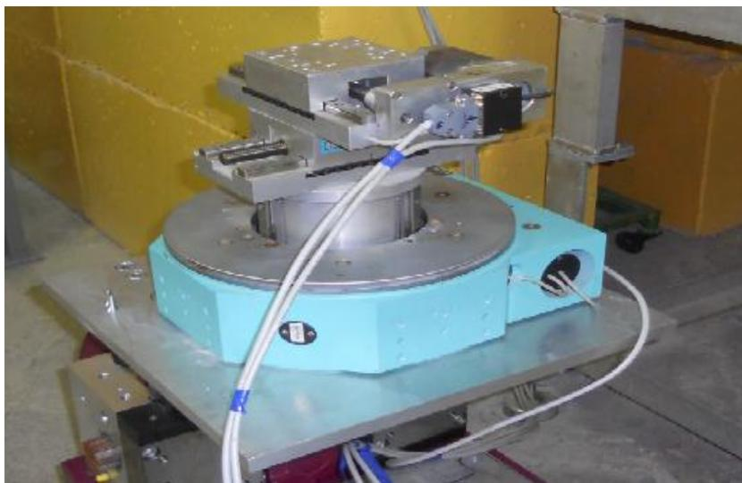
**Fig. 6.4.** Huber goniometer of the FSS spectrometer.
