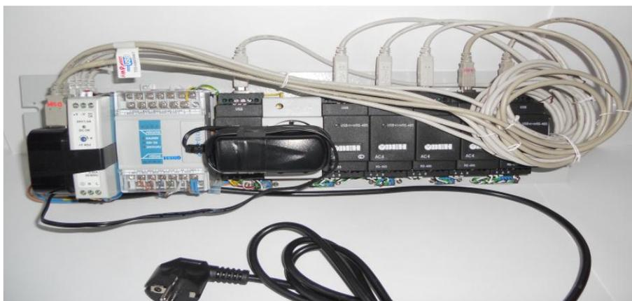
**Fig. 6.5.** Control system on the basis of AS4 (USB-RS485) and AC3-M (RS485-RS232) interface converters.
