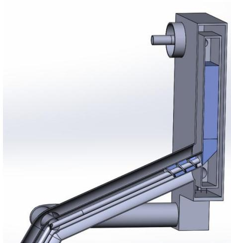
**Fig. 1.4.** Screw-type discharging device (model).
