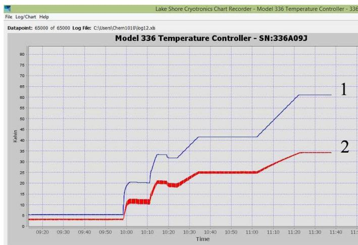
**Fig. 4.6.** Time dependence of temperature of sample chamber as temperature changes: 1 – temperature of sample chamber, 2 – temperature of cryorefrigerator second stage.
