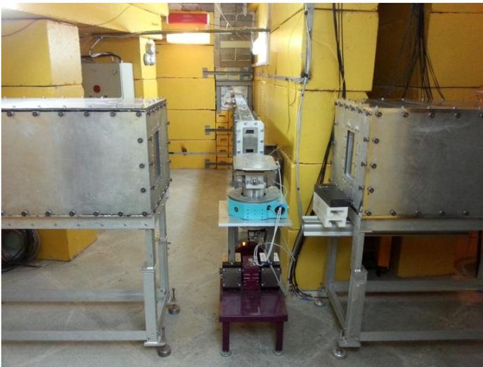
**Fig. 3.5.** A sample table with a goniometer and 90° scintillation detectors "Ost" and "West" on IBR-2 beamline 13.
