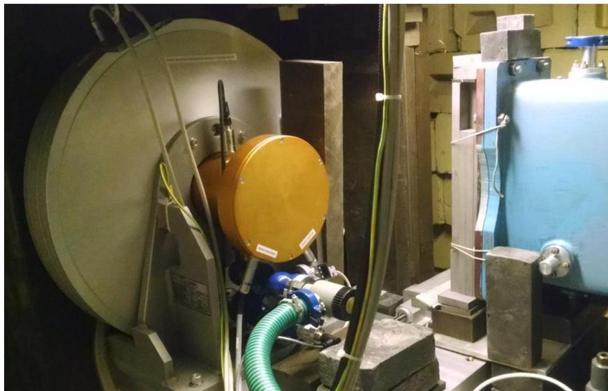
**Fig. 6.8.** Fourier-chopper on HRFD diffractometer.
