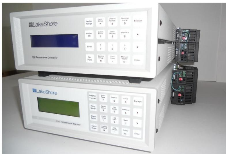
**Fig. 6.6.** LS325 controllers after modernization.
