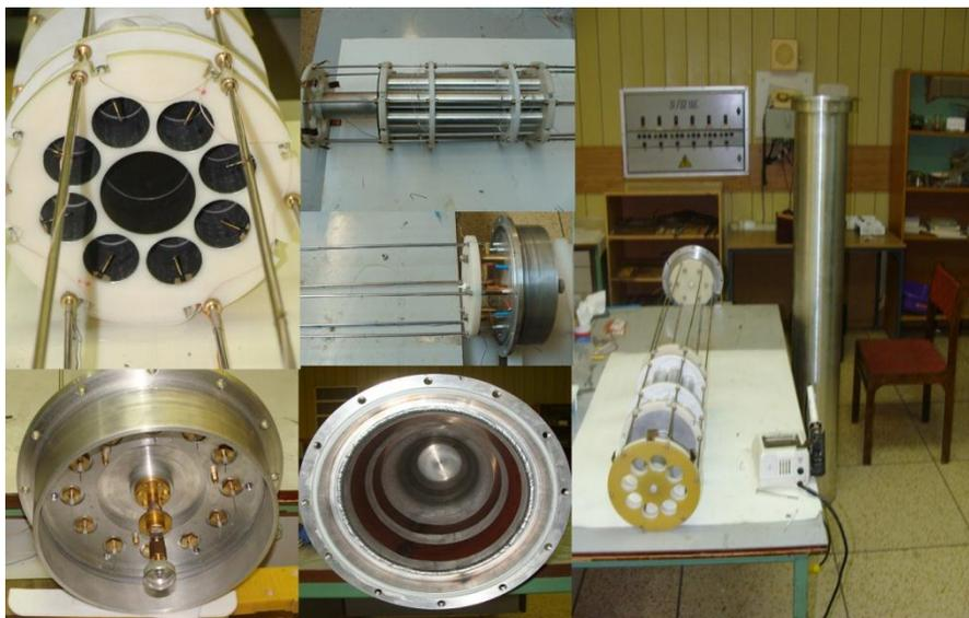
**Fig. 5.3.** Housing and electrode system of recoil proton telescope.
