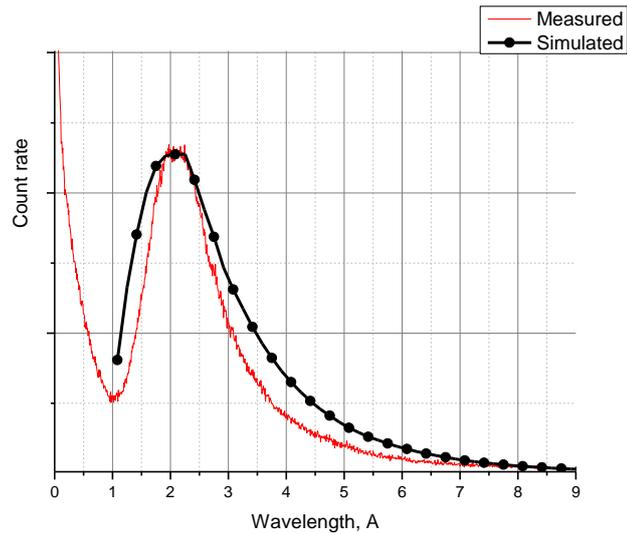
**Fig. 3.4.** Calculated and measured distributions of neutron beam intensity at the exit of the mirror neutron guide.
