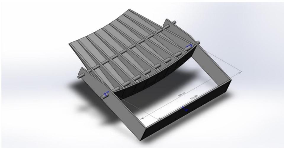
**Fig. 5.10.** 3D model of one of the planes of the new ASTRA-M detector.
