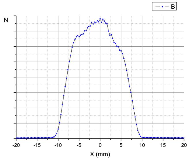
**Fig. 3.3.** Distribution of beam intensity along the x-axis at the exit of the neutron guide.
