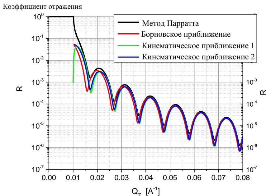
**Fig. 2.3.** Simulation of specular reflection for the system presented in Fig. 2.1 using various methods.
