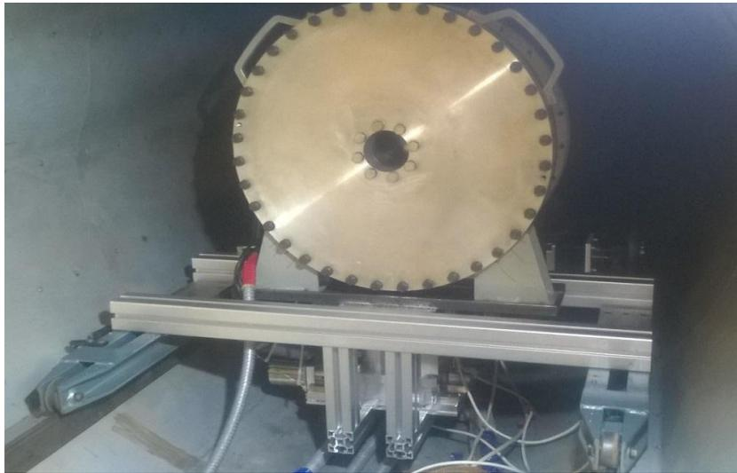
**Fig. 6.3.** Platform with a detector mounted on the position adjustment mechanism for moving in the horizontal and vertical directions.
