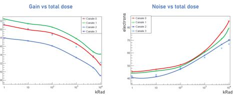
Gain was calibrated with <sup>55</sup>Fe source [Left, signal and noise for the SEED 4 quadrants, featuring different CE geometries]. The gain is only slightly affected up to about 1 kGray (100 kRad). TID is done using x-rays (Seifert machine).
