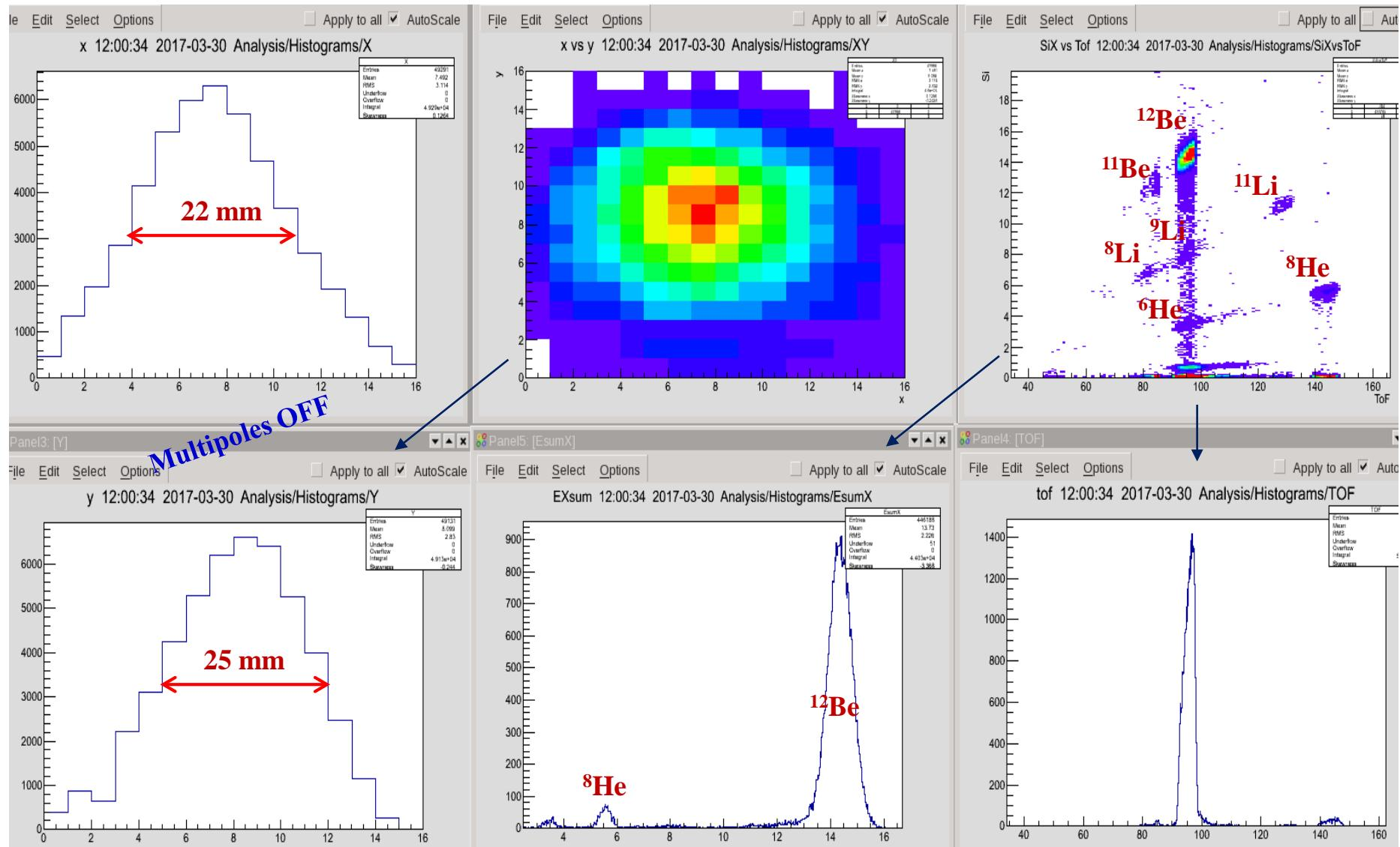
**${}^6\text{He}$  from  ${}^{15}\text{N}(49.7 \text{ AMeV}) + \text{Be}(2 \text{ mm})$ :**
