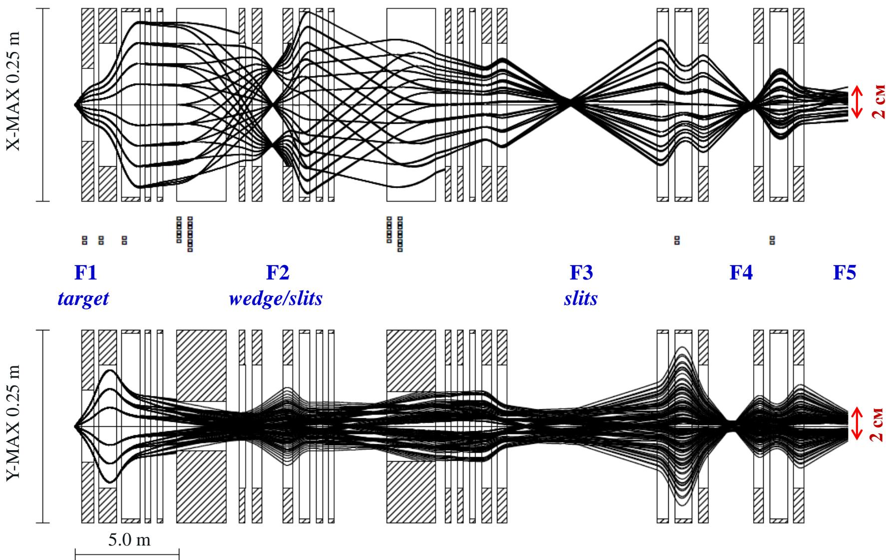
**RIB's profile estimation in  $^{15}\text{N}$  (49.7 AMeV) + Be (2 mm) reaction
