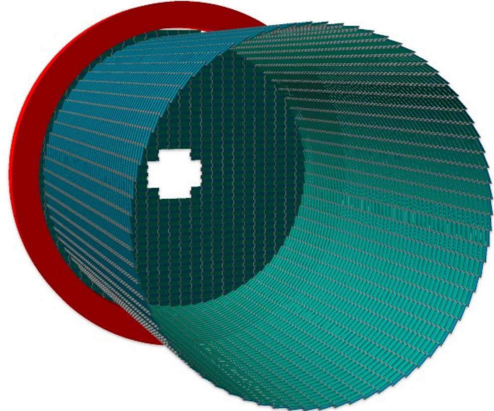
Figure 4.35: Two technologies are being considered for the time-of-flight system of SPD: the multigap Timing Resistive Plate Chamber, mRPC (left) and the plastic scintillator option (right). Barrel and one of two end-cap parts are shown for both options. One of six magnet coils limiting the volume of TOF is shown in red.
