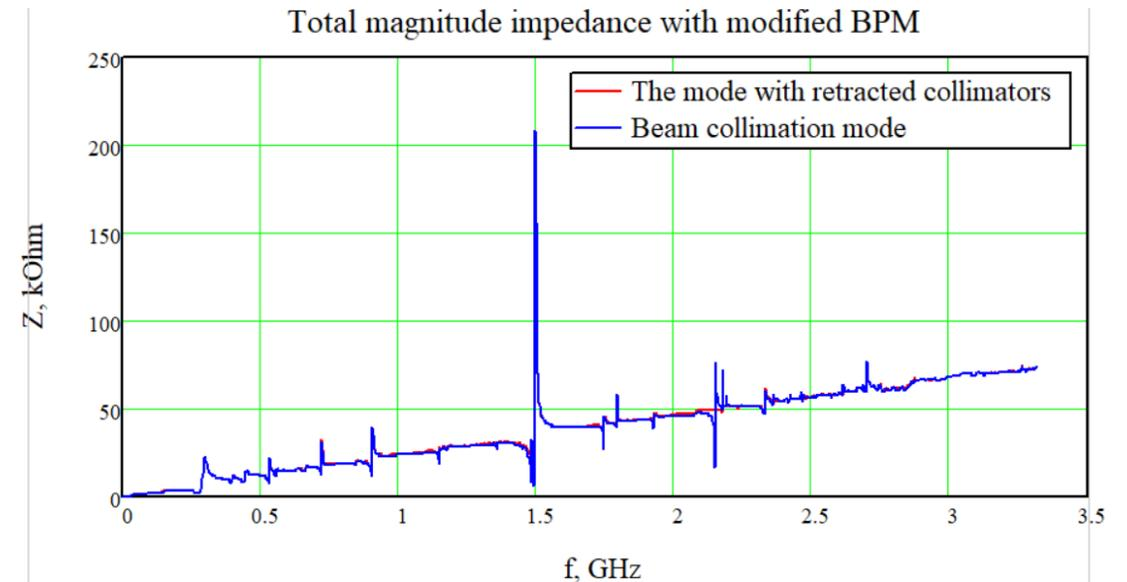
*Total magnitude impedance with initial (left) and modified BPM for the mode with retracted collimator (red curve) and beam collimation mode (blue curve).*
