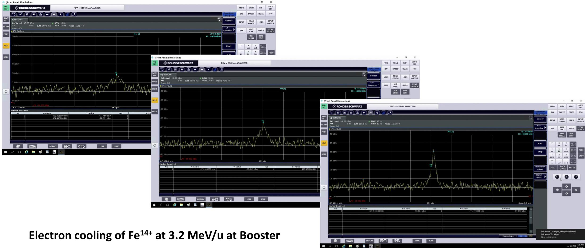
Electron cooling of Fe<sup>14+</sup> at 3.2 MeV/u at Booster
