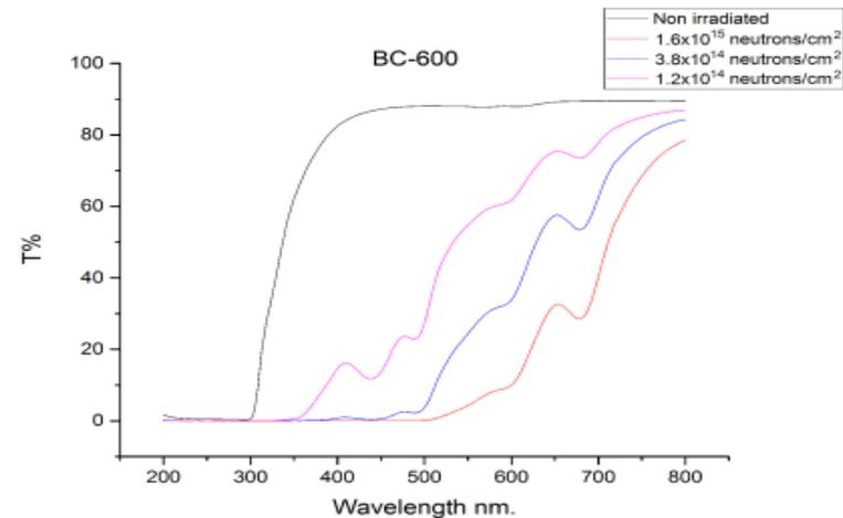
Transmission spectra of glue SKTN-MED(D) (a), BC-600 (b) measured on neutron integral flux ( $1.6 \times 10^{15}$ ,  $3.8 \times 10^{14}$ ,  $1.2 \times 10^{14}$ ) neutrons/cm<sup>2</sup>
