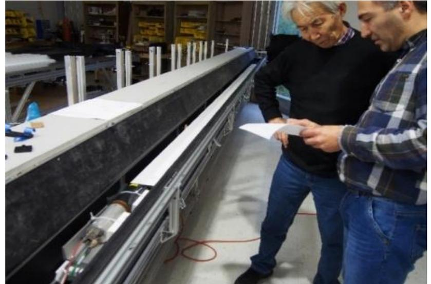
In the 2015,2016 a group of JINR colleagues was sent to the University of Virginia, USA to establish a mass-production process of scintillation modules CRV. They successfully develop a procedure of module assemble and created two pilot CRV modules with a length of 90 cm and prepared scintillation strip components for 4.5 meter length module.
