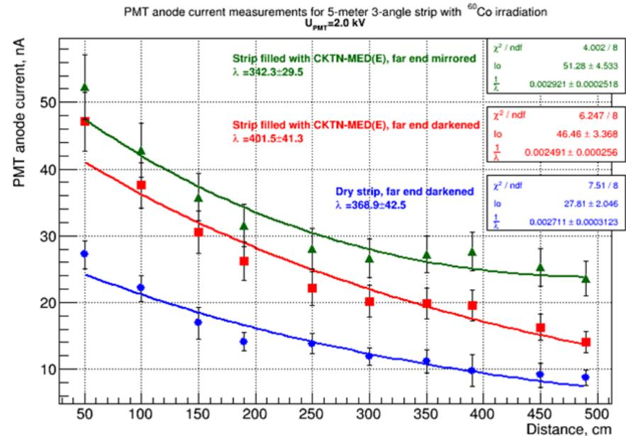
Light yield collection for the strip filled by CKTN-MED(E) with 1.2 mm WLS fiber.
