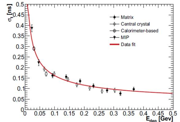
Time resolution as a function of the energy deposited in the matrix
