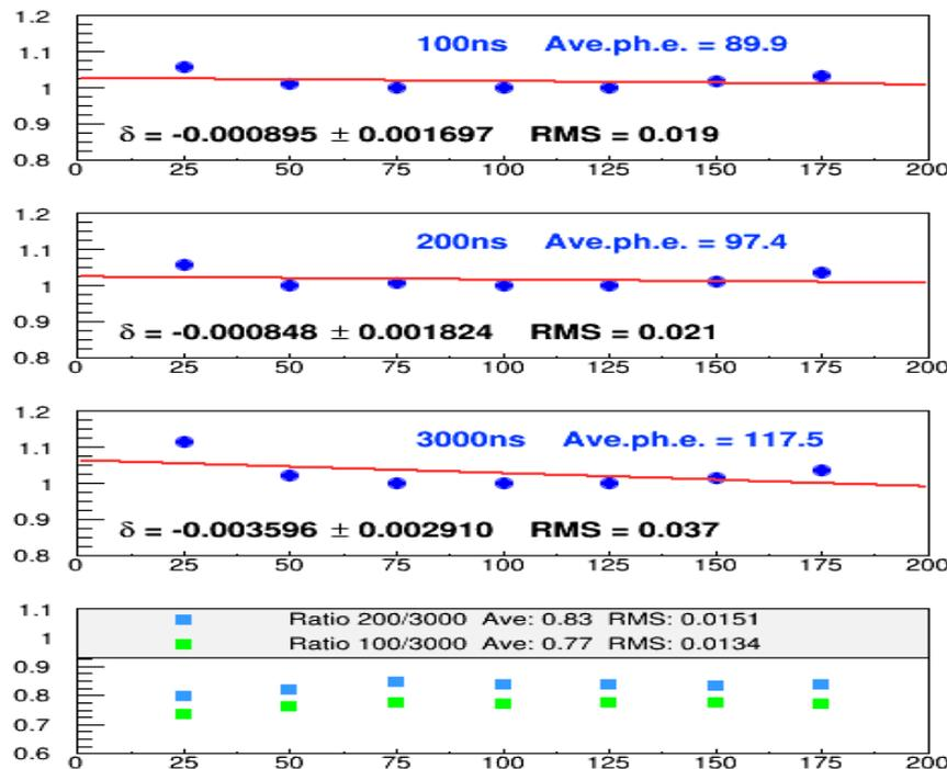
Longitudinal response uniformity and ratio fast to total scintillation component
