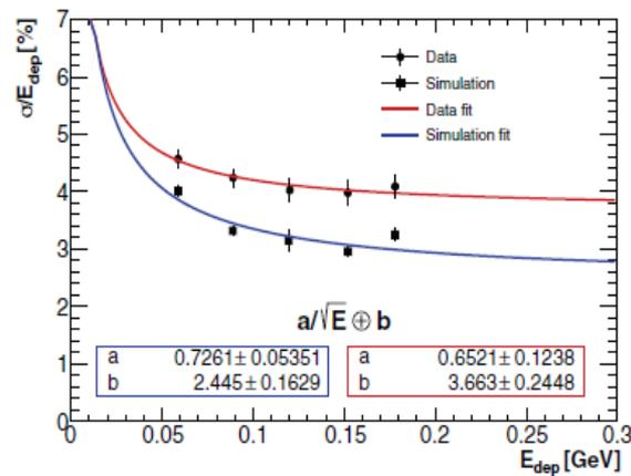
energy resolution as a function of the deposited energy
