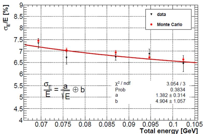
Figure : Energy resolution obtained from the data (black) compared with the Monte Carlo (red).
