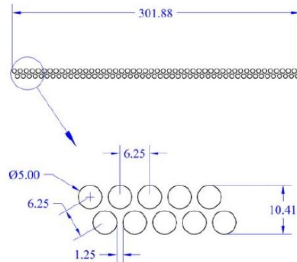
Figure 8.7. Edge view of a panel showing the arrangement of straws within a panel. Dimensions are in millimeters.
