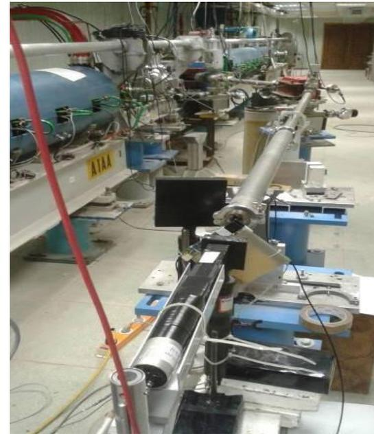
We investigating the possibility to obtain of a low-intensity (1...3 electron) beam of elections at the linear accelerator LINAC-800. Low-intensity beam of electrons with 1...3 electrons on each spill will allow us to study the characteristics of CsI and other type crystals.
