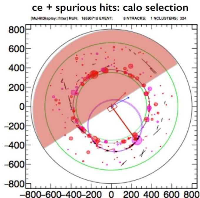
Example of a full simulated conversion electron (CE) event in overlap with all hits from the environmental background: (left) without any requirement on the calorimeter system and (right) with a calorimeter based selection. Black points are hits from the tracker. Red points are from calorimeter clusters. By requiring the track hits to be in time with the most energetic cluster of the event, in a time window of 50 ns, the quantity of background hits is strongly reduced
