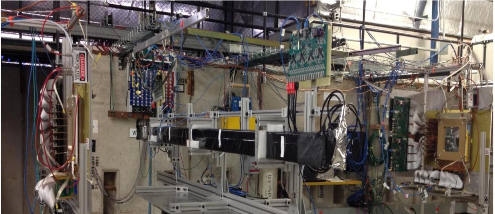
Tests of the CRV counter prototypes were performed at Fermilab 120 GeV proton beam.
