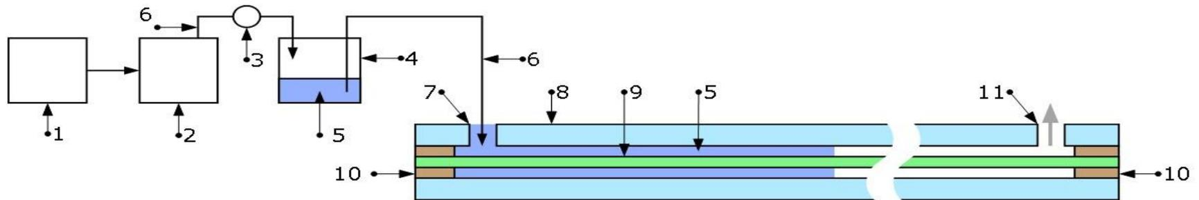
Figure. Setup to pump the high viscosity filler into the co-extruded hole of the scintillation strip (not in scale): (1) dry type compressor; (2) SL101N digital Liquid Dispenser; (3) manometer; (4) special vessel with filler; (5) filler; (6) polyvinylchloride tube; (7) inlet for filling; (8) strip; (9) WLS fiber; (10) sealing; (11) exhaust outlet for extracting air.
