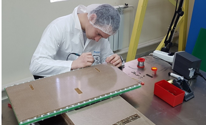
Soldering HV connector and readout pins
