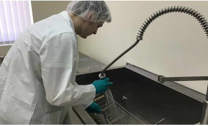
Glass cleaning with ultrasonic wave & deionized water
