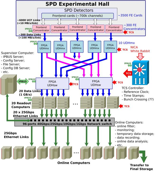
CDR version of DAQ based on ideas and hardware developed by I.Konorov for COMPASS/AMBER experiment
