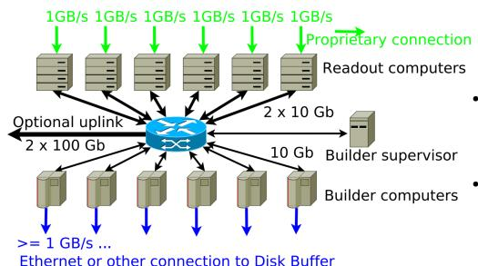
The contiguous set of slices (chunk) or the full frame containing data from all detectors are bullied by the pool of Builder computers under control of the Builder supervise.
