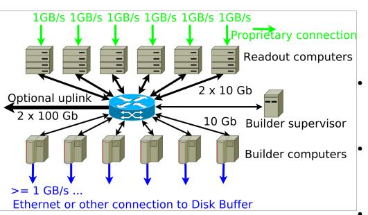
The contiguous set of slices (chunk) or the full frame containing data from all detectors are bullied by the pool of Builder computers under control of the Builder supervise.
