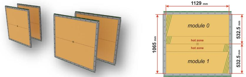
Configuration of the CSC detector for RUN-8
