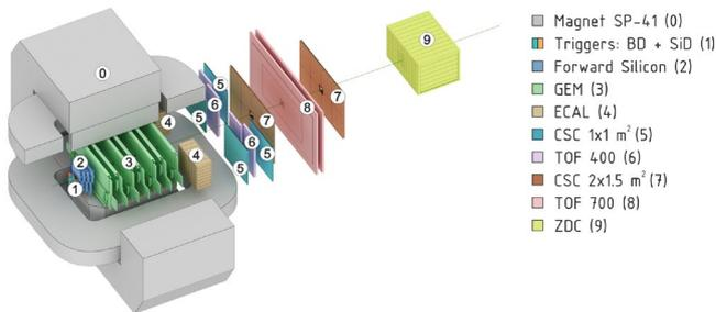
Configuration of the BM@N setup for the first experimental run in 2022
