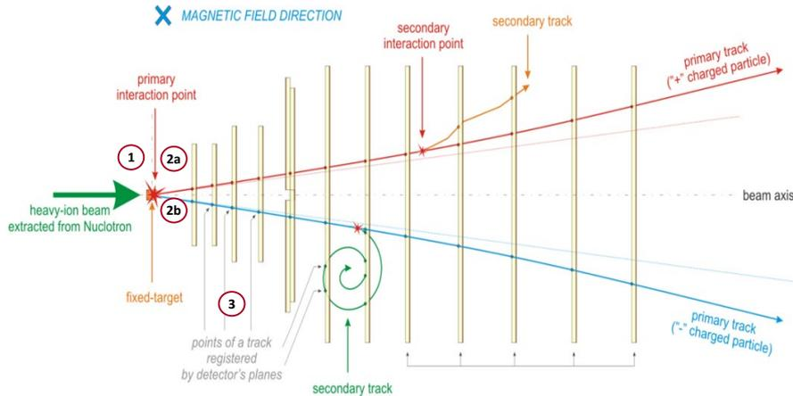
1. A heavy-ion beam, extracted from Nuclotron, collides with a fixed target
