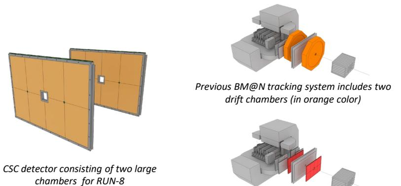
CSC detector consisting of two large chambers for RUN-8
