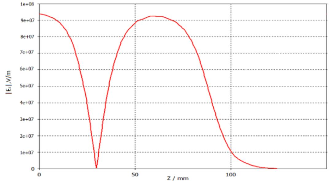
Figure 3: Dependence of the amplitude of the accelerating field on the axis of the cavities on the longitudinal coordinate.
