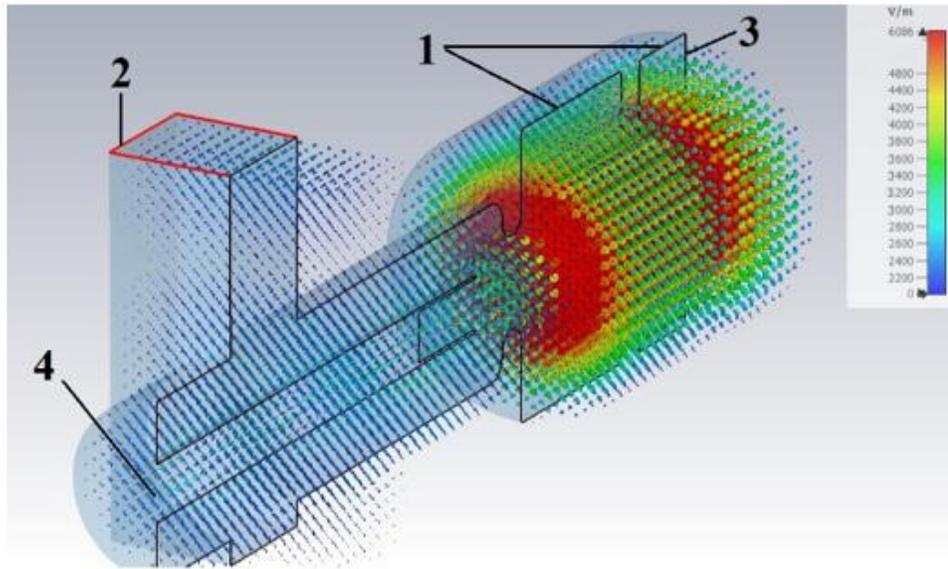
Figure 2: RF photogun layout (1-accelerating cavities; 2-RF power input; 3-cavity wall with a photocathode; 4-cavity for laser input and beam output).The electric field in the accelerating cavities corresponds to an input microwave power of 4 MW.
