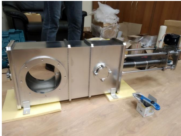
Vacuum box for Ion beam profile meter. Detector movement range is 30 cm
