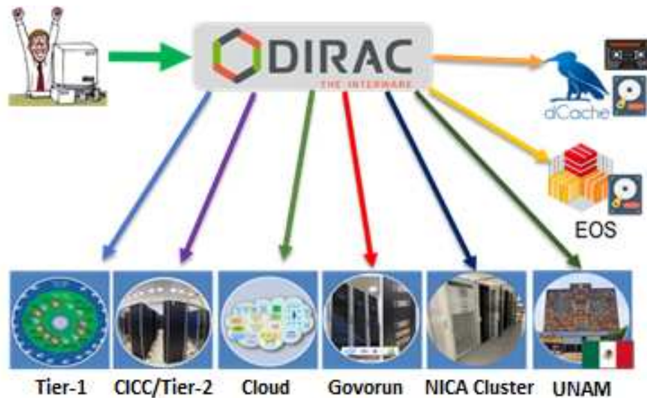
Fig. 2. Scheme of the integration of geographically distributed heterogeneous resources based on the DIRAC Interware
