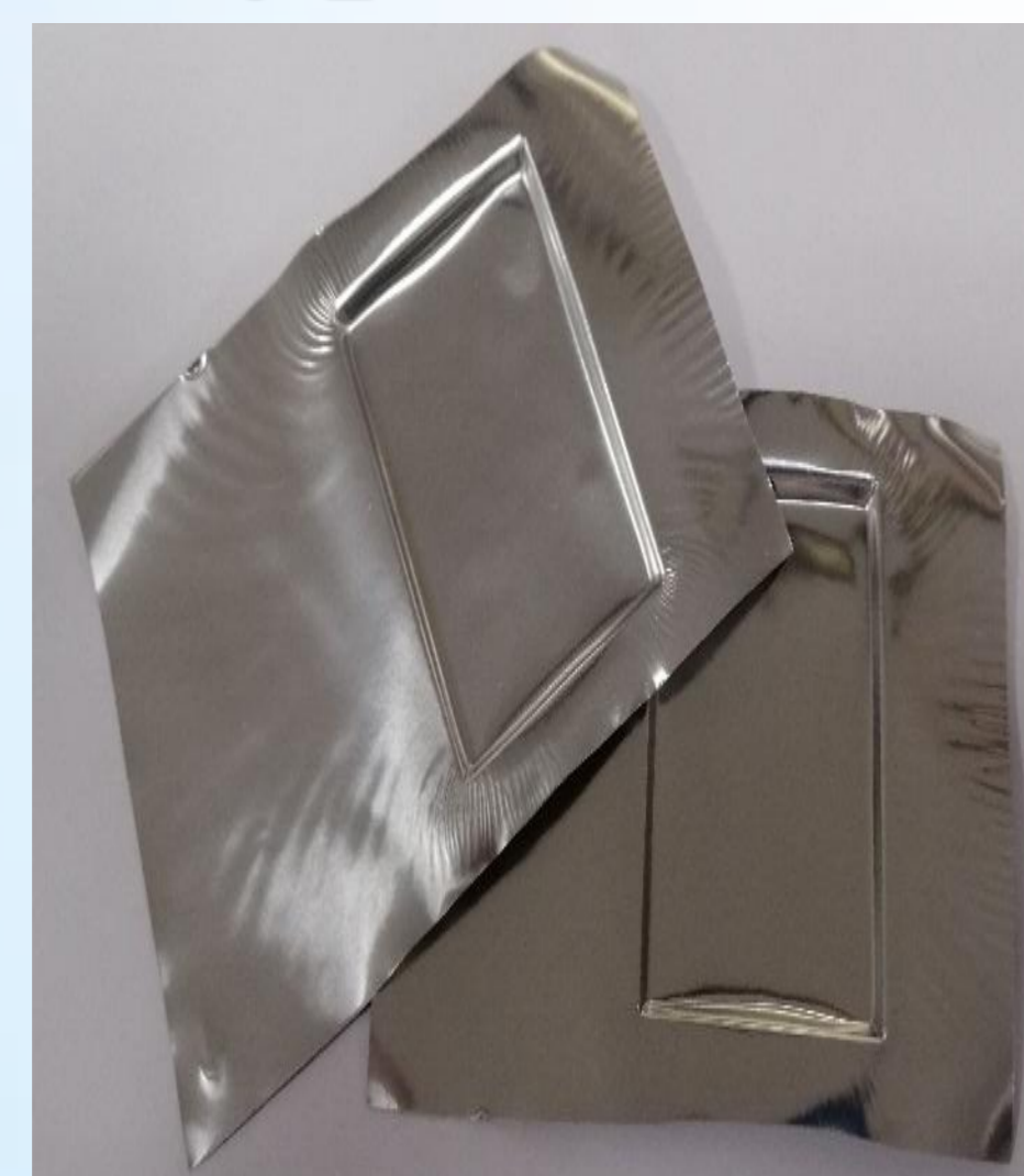
Figure 5. pouch cell case parts
