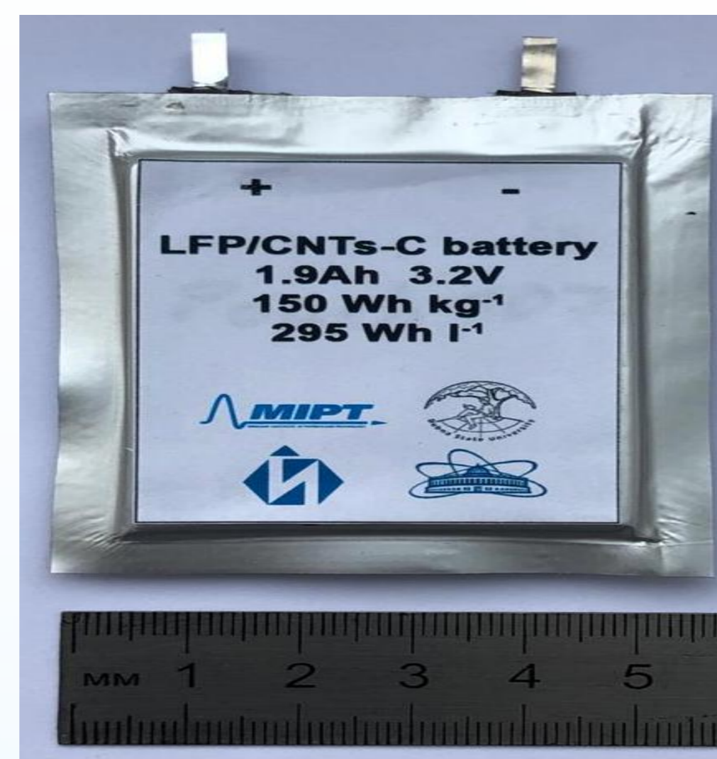
Figure 6. pouch cell after the formation and re-sealing
