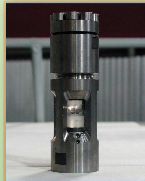
High-pressure cell with sapphire anvils
