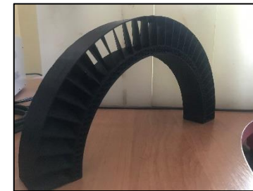
Fig. 9-10. The general scheme and the printed part of the optional velocity selector for VCN. It may be able to be used instead of the proposed chopper system.
