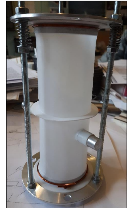
Fig. 11. The first example of the PTFE cylinder with the converter tube.
