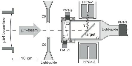
PSI:  $\mu$ E4 beam-line Number of  $\mu$ -stop = (8 - 25) x 10<sup>3</sup> with 20 - 30 MeV/c
