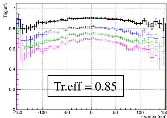
FHCAL trigger efficiency vs. z-vertex
