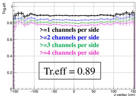
FHCAL trigger efficiency vs. z-vertex
