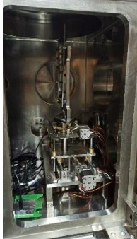
a) The system for online diagnostics and control of peripheral ion flux density and fluence
