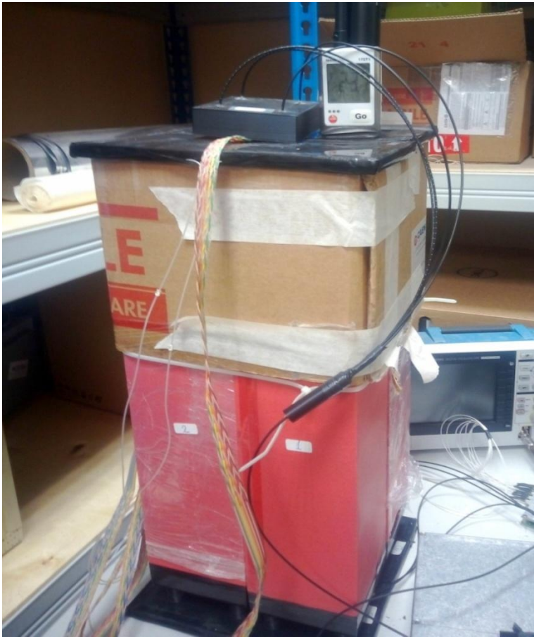
Figure 13: Photo of the calorimeter test setup consisting of 4 modules of the size 11 \times 11 \text{ cm}^2 , with the total cross-section of 22 \times 22 \text{ cm}^2 . The environment temperature was measured by thermistors, provided for each 4 MPPCs board and by digital thermometer as well. One of the boards in light protection cover and the digital thermometer are placed on the top of the setup. The optical fibers (visible on photo in Fig. 13) distribute the light from LED generator.
