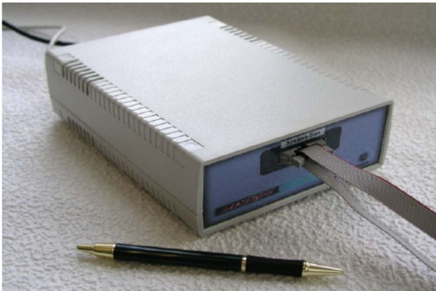
Figure 12: Control power box (HV) for MPPC bias Voltage.
