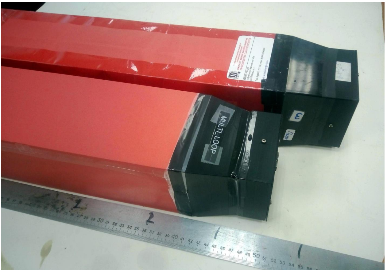
Figure 7: Two calorimeter's modules covered in light isolation paper are shown in this photo. The modules have different length due to different layers number 190 and 220 and different absorber thickness 0.5 and 0.3 mm correspondently.
