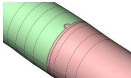
Design of the non-flange connections (Butyl rubber sealing tape)
