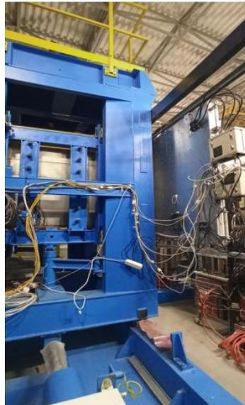
FHCAL and scWall installed at the BM@N
