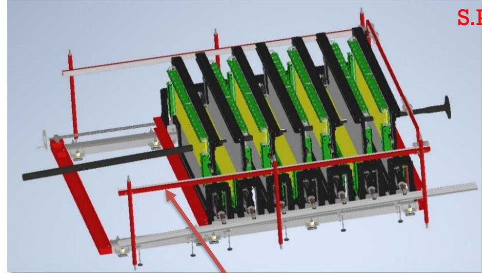
GEM support mechanics inside the SP-41 magnet. Red parts are needed only for installation and will be removed afterwards.
