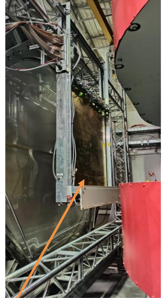
Three CSC chambers are installed into the SRC setup
