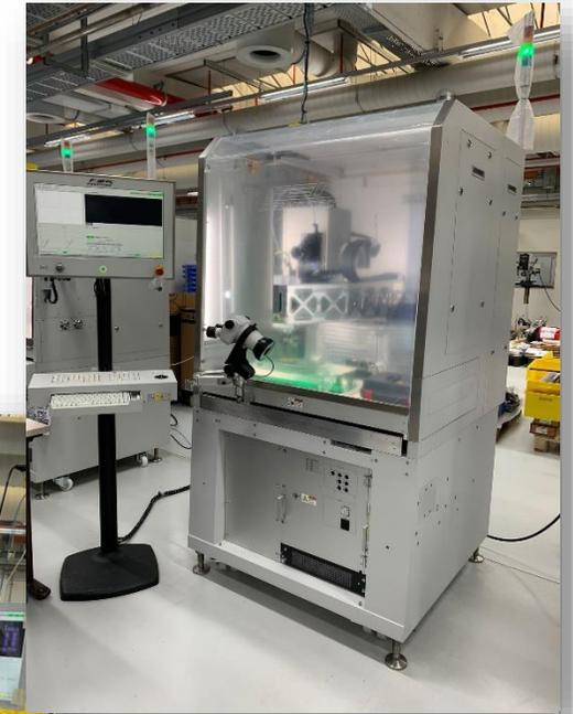
New ultrasonic bonding machines for the serial production of modules
