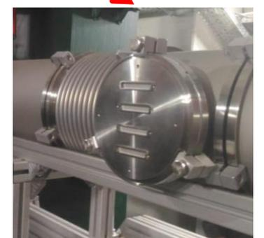
The beam pipe, vacuum boxes and target station are ready. The design and production of the target station control system and pneumatic actuator mechanics was performed by A.Kubankin group.
