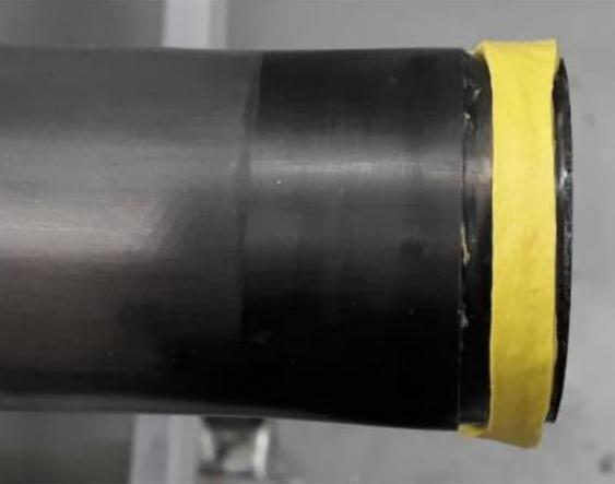
The tape is carefully compressed around the surface to avoid the unsealed zones
