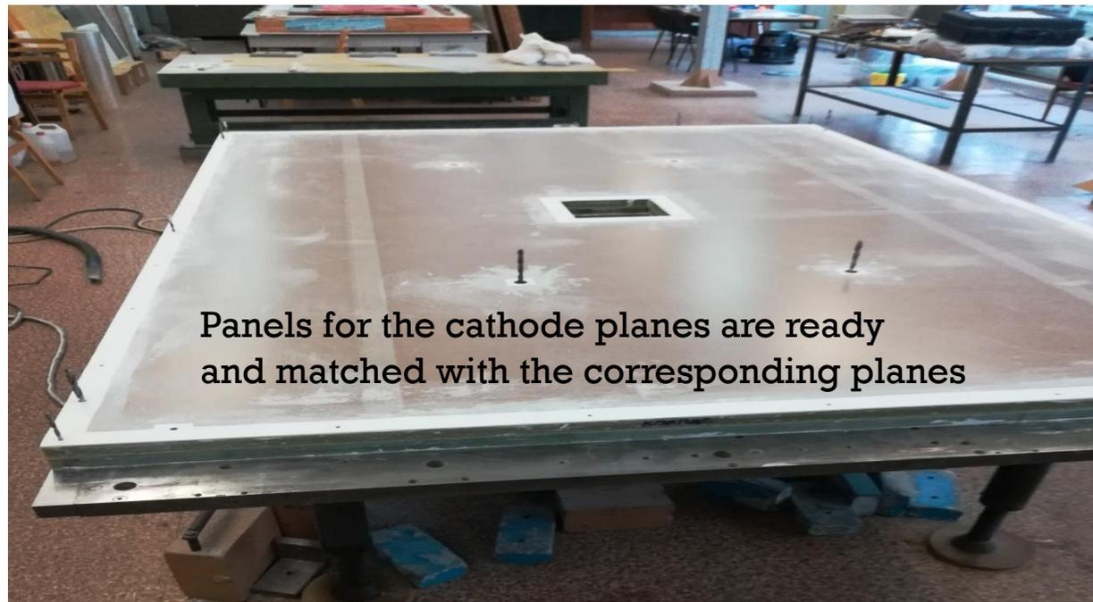
Panels for the cathode planes are ready and matched with the corresponding planes
