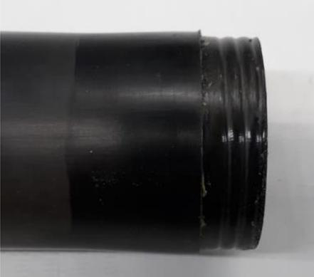
The connections are cleaned before sealing
