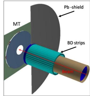
Simulation of  $\delta$ -electron background for different thickness of inner shield
