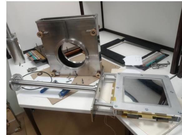
Ion beam profilometers. Effective area 80x80 mm<sup>2</sup>, 128x128 mm<sup>2</sup> and 192x192 mm<sup>2</sup>.
