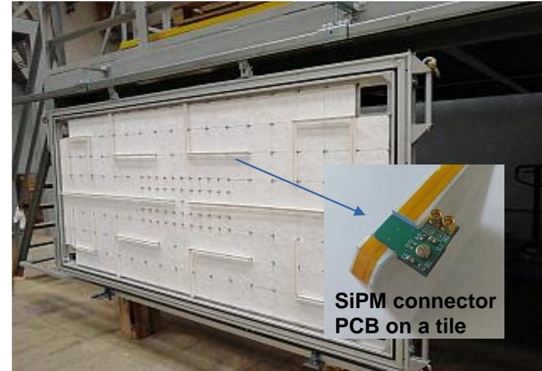
Scint. Wall fully equipped with tiles (for tests at INR)
