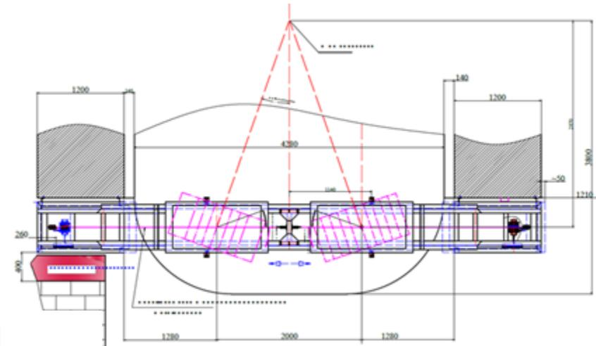
The calorimeters are located between the coils of the SP-41 magnet directly behind the GEM chambers.
