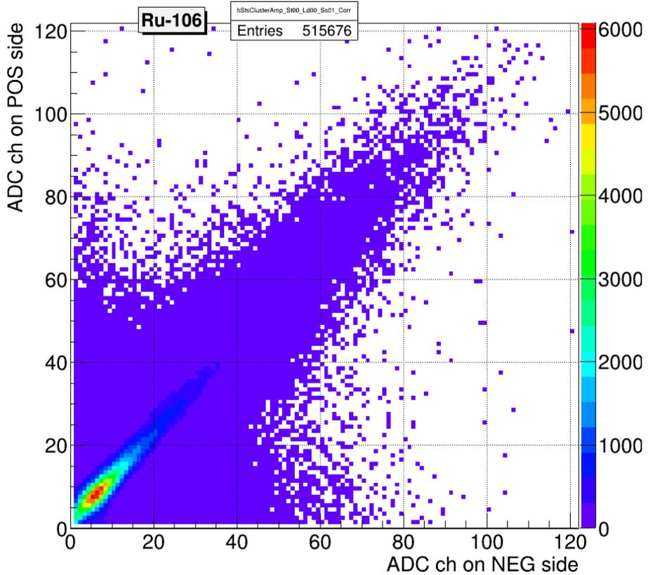
Measured signal from the Ru-106 radioactive source
