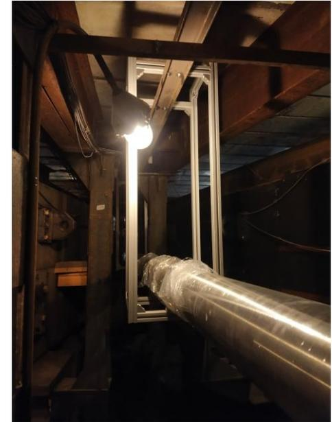
Vacuum tests of the assembled beam pipe –  $10^{-6}$  Torr
