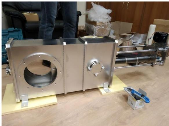
Vacuum box with the beam profilometer: two positions of the profilometer. Travel range is 0-300 mm.
