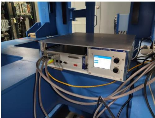
WIENER MPOD power supply unit has been installed
