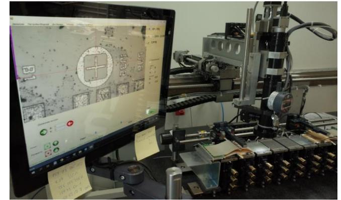
Measuring of the sensors positions on the ladder
