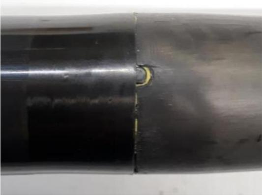
After preliminary vacuumization spare tape is removed
