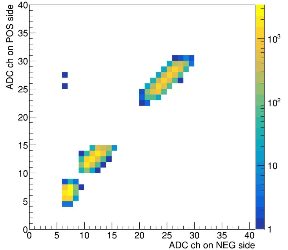
Measured signal from the IR laser (three different amplitudes of laser pulses)
