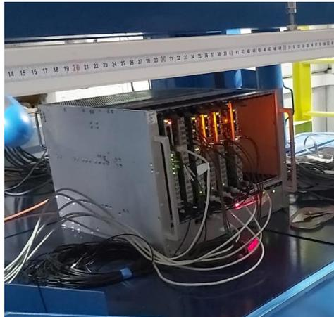
VME crate for beam hodoscope installed on FHCAL platform
