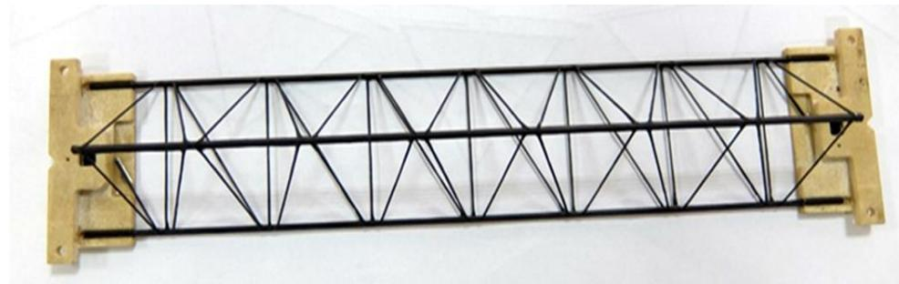
CF-truss with bearings
