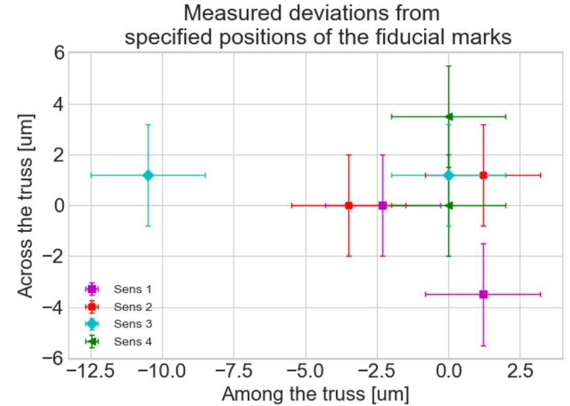
Each sensor has fiducial marks on its surface. Position of each mark is specified for each module on a specific ladder.
