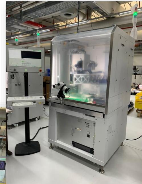
**New ultrasonic bonding machines for the serial production of modules**
