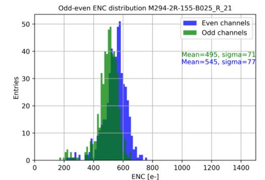
Measured noise per channel distribution for the module on ladder
