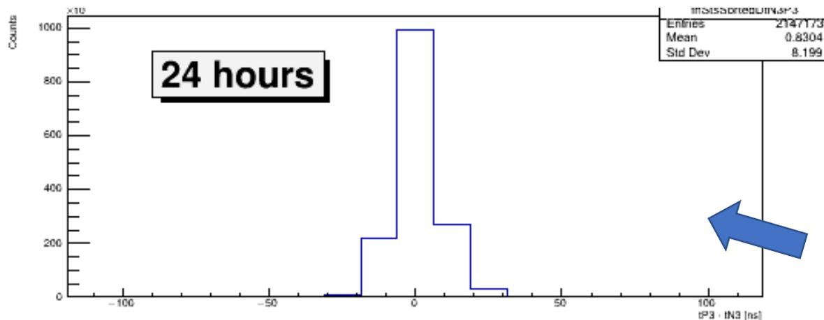
Measured time difference in ns between hits on the P and N sides of the sensor
