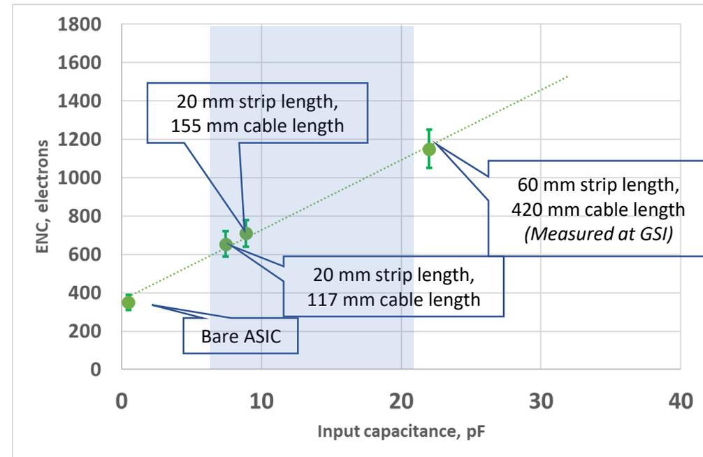
Noise level depending on the type of the module (sensor size and cable length)
