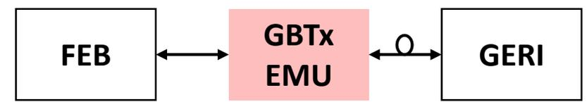
The GBTxEMU board is prepared as a controller and data concentrator of BM@N STS module readout chain
