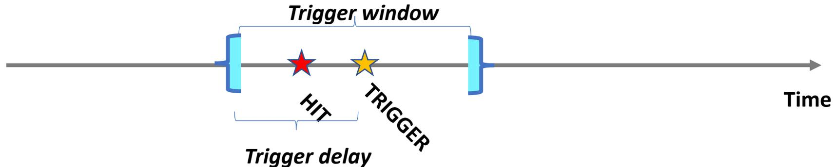
Trigger window and trigger delay parameters could be configured within the specified range:
