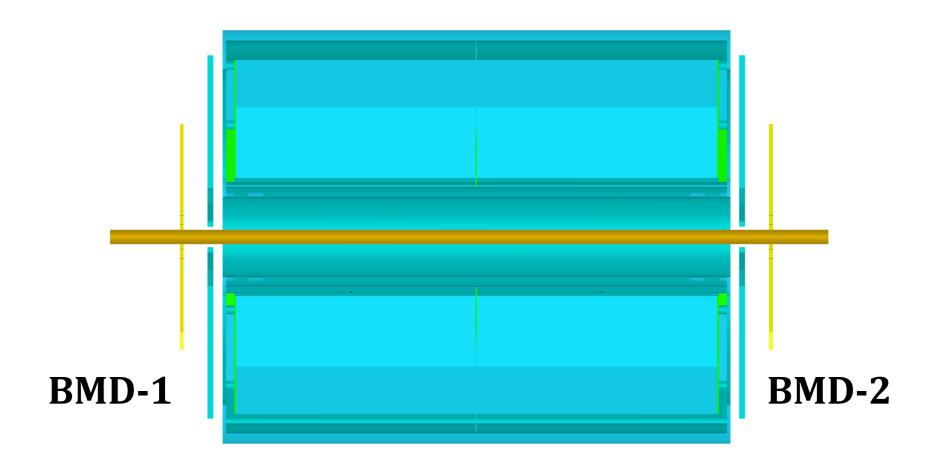
As a first approach, the BMD system will consists of two detectors located at 2 meters away from the interaction point of the MPD-NICA, BMD-1 and BMD-2 respectively. Each detector is composed by an array of 80 cells made of plastic scintillator arranged in five rings forming a sixteen sectors disk of 153.26 centimeters of diameter. The pseudorapidity coverage of BMD would be  $1.69 < |\eta| < 4.36$ .
