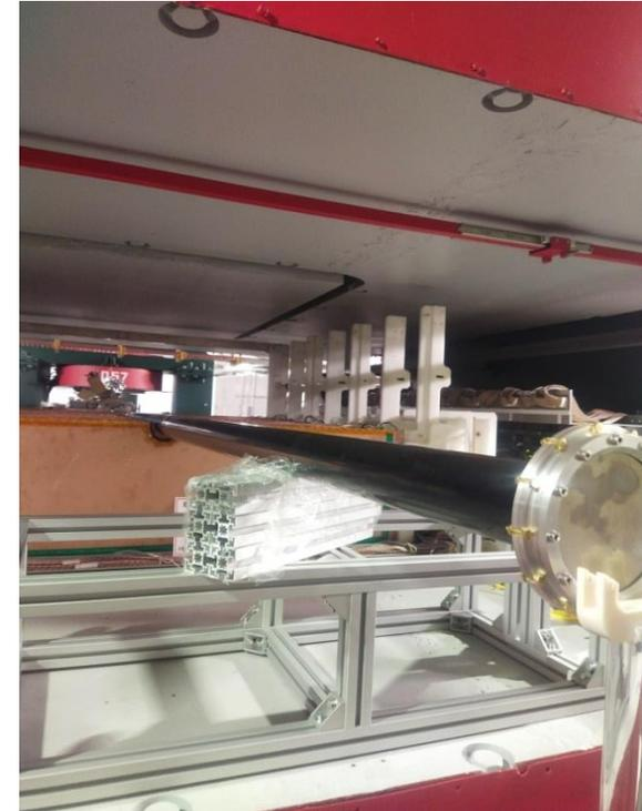
The moment of adjustment of the carbon beam pipe
