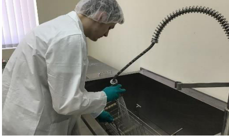
Glass cleaning with ultrasonic wave & deionized water
