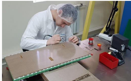
Soldering HV connector and readout pins
