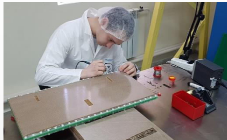
Soldering HV connector and readout pins
