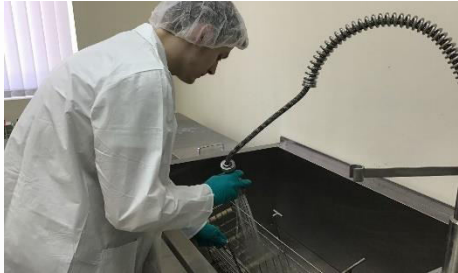
Glass cleaning with ultrasonic wave & deionized water
