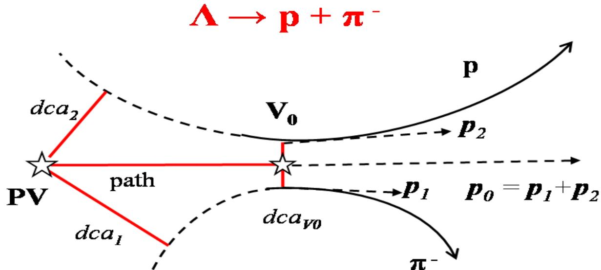
**Event topology of two-particle decay of the neutral particle:**
