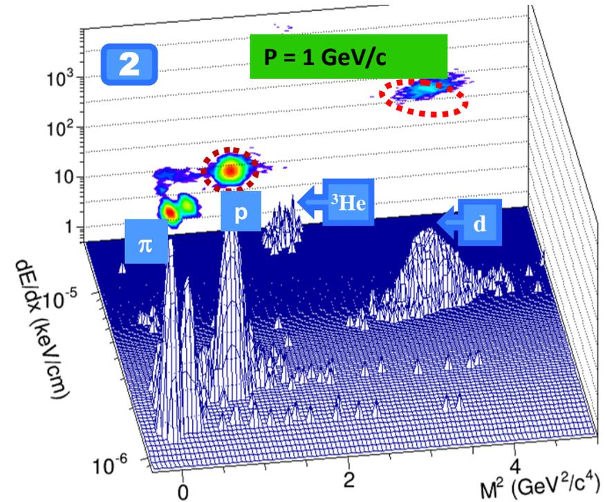
Particles are selected within  $3\sigma$  cuts in ' $dE/dx$  vs  $p$ ' (1) or ' $dE/dx$  vs  $m^2$ ' space in momentum bins (2)
